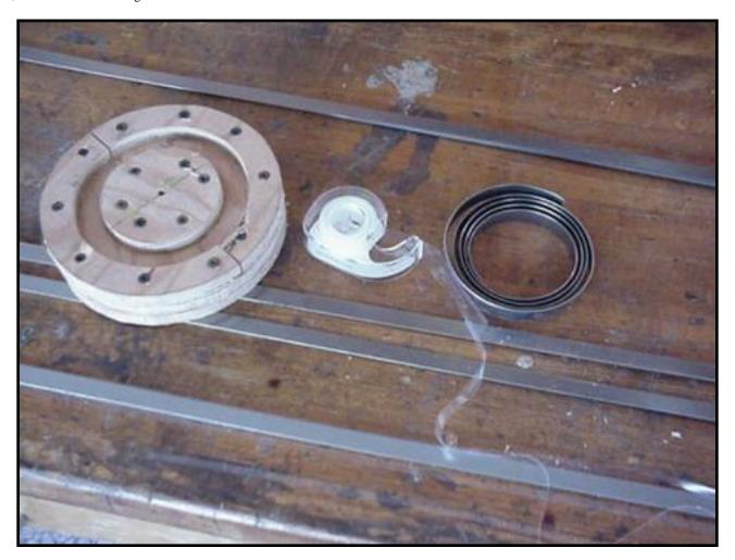
Show above is the plywood stator, glued, and screwed together. You can clearly see the cavity into which the laminates will be glued in. The laminates are made up of 1/2" wide strips of 20 gage cold rolled steel sheet metal. The strips I used are 4' long, and before installing them, I covered 1 side of each strip with tape so that each piece would be insulated from the one beside it! This is very important to reduce eddy currents.
