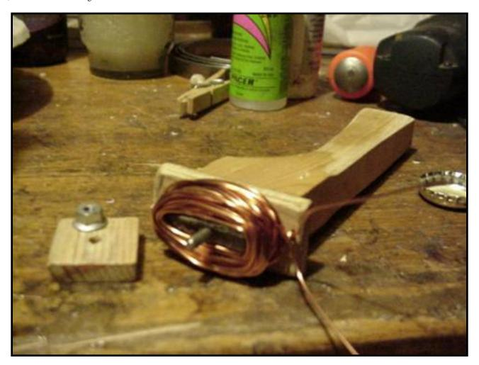
Above is shown the same coil winder with a finished coil on it. Each coil is made up of 40 turns of AWG 18 magnet wire. Once the coils are finished, I twisted the ends tightly together before removing them from the winder.
