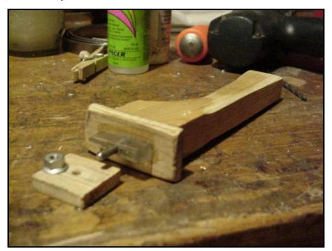
The coils are glued (with epoxy) on top of the stator - right over the top of the steel laminates. Before making the coils I made a very simple winding form - simply a handle, with a small plexiglass form on top (where the coils would be formed), and a cap, which is held on with a nut. I could hold it in one hand, wind the coils with the other, and when the coil is done the top is removed so the coil can slide off.
