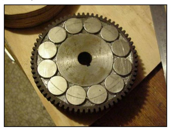
I cut a slot in the gear 1" wide, and about 1/8" deep to hold the magnets in. The magnets must be evenly spaced around the circle, and once they were, I glued them in with epoxy. This is very similiar to the Volvo disk brake alternator I made - so check that page out for more detail. The polarity of the magnets around the circle alternates, so each magnet has the opposite pole up as its neighbor.
