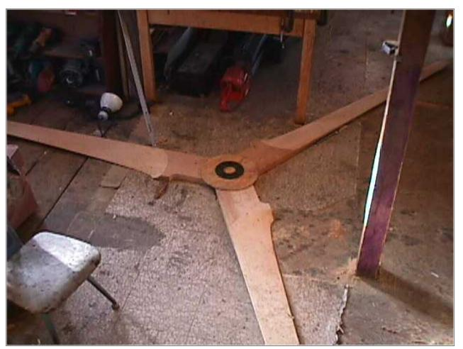
Here are my 14' blades on the floor of my shop. They are made from nearly perfect and expensive vertical grain fir, not a knot to be found. The blades are much too large to assemble and get out my door, so I had to assemble them on the floor, mark things out, drill the holes for the studs in one blade at a time, and then assemble them outside.
