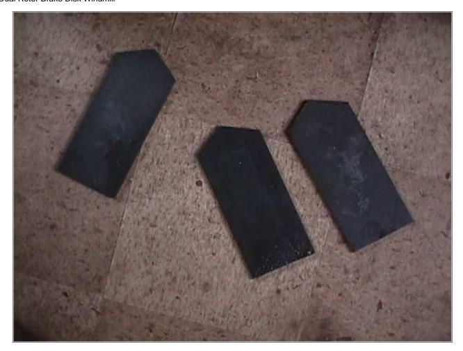
Since this is a dual rotor machine, the stator will not be able to bolt on in place of the backing plate like I've done in the past. The stator will have to be in between two rotors, and held on by a bracket which ties into the outside of the stator. These are the pieces I made up for this bracket. The bracket will actually bolt on in place of the backing plate (to the strut assy behind the wheel spindle). These 3 pieces are cut from 3/16" thick X 3" wide steel, and they are 7" long.
