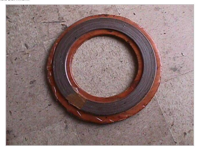
Probably not necessary, but I glued the steel laminates into a plywood ring to make them easier to handle and prevent corrosion.
