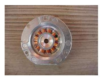
The inside layout of our tiny Brushless PM DC Motor looks just like the Wood 103's alternator!
