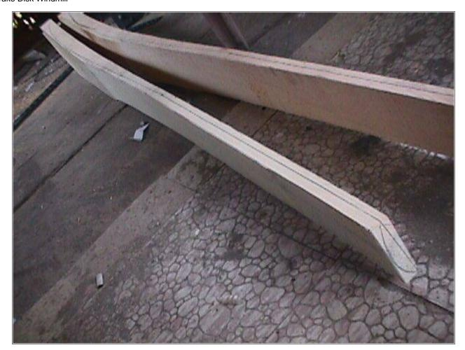
These are simple blades (as usual with me...). The tips are pitched about 4 deg, and the middle of the blade about 6 deg. From there it pitches steeper and steeper until the angle takes up the board thickness near the root of the prop. The airfoil is designed to do little more than 'look like an airfoil' and the thickest part of the airfoil is about 1/3 of the way back from the leading edge towards the trailing edge.
