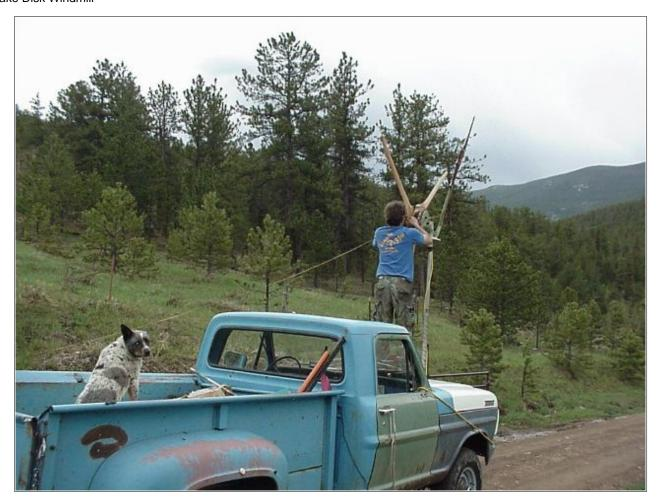
In this picture I'm tying it up so we can more easily navigate the trees on our driveway for the ride home. This picture does give a good idea of how the furling system works, as the wind puts force back on the blades it makes the machine want to fold up like this - but in order to do so the tail must be raised! So the furling system is a balancing act between the force back on the blades, and the weight of the tail.
