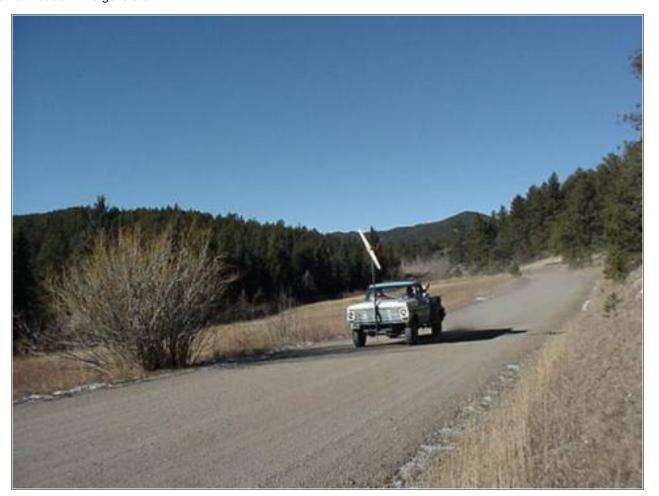
To test it we simply put it on the mast which I keep mounted to the nose of my '70 F250 and go driving on a still day! We had wonderful results when we tested this, all of our test results came out very consistant - they all fall exactly on a nice curve which we plotted on graph paper. In the truck, we carry a 12 volt battery, a volt meter, and an ammeter. We watch the speedometer, vs system voltage (between 12-15 volts volts when charging) and the ammeter. Here is the bottom line...
