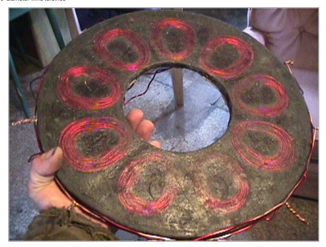
The stator came out pretty well. We cast these with polyester resin, the sort you buy at an autoparts store for fiberglass layup. There is a layer of fiberglass to reinforce the stator on each side of the coils.
