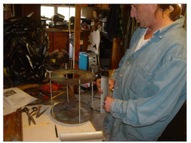
We put 10" between the two sides of the runner using allthread, and squared it up as best we could before installing the vanes. You can see some of the holes we drilled to help with postioning the vanes.
