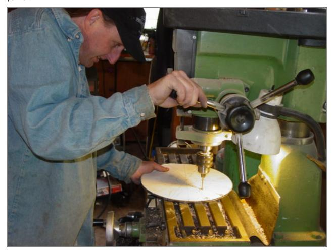
The template is glued to one of the disks which make up the sides of the runner, and we have both disks clamped together. Pictured above we're drilling small holes which will help us know exactly where to postion the vanes.
