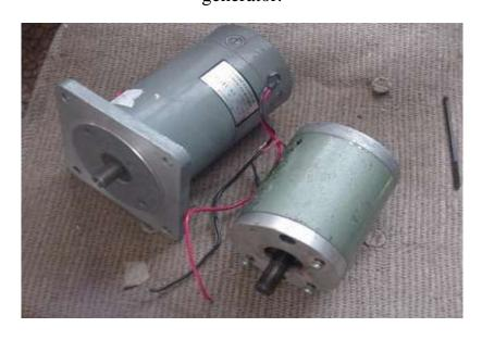
Surplus tape drive motors can make a quick and easy generator for small windmills
