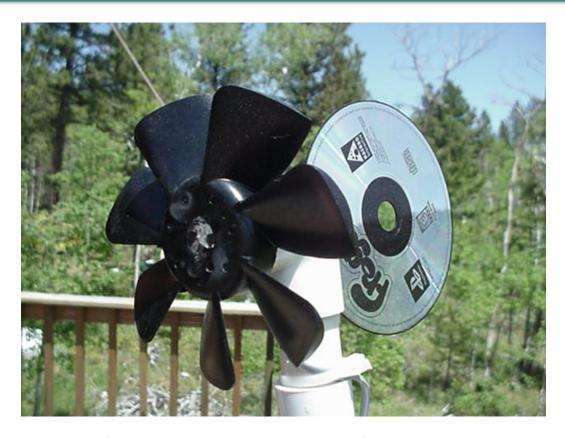
The frame is made of PVC pipe, the tail from a video game CD, and the rotor from a computer fan. The generator is a small DC hobby motor. It will light a small bulb using an electric window fan for power.
