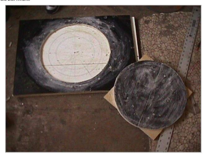
I made a mold out of partical board. The circle is 14 inches in diameter and I divided it into nine parts and drew lines so that I know where to place the coils. The top of the mold is the cutout from the bottom. The mold is 1/2 inch thick. I waxed the mold so that the resin would not stick to it. Once I place the coils and pour the resin, the top will get clamped in, and the wires from each coil will poke out the edge so all the wiring will be done later.
