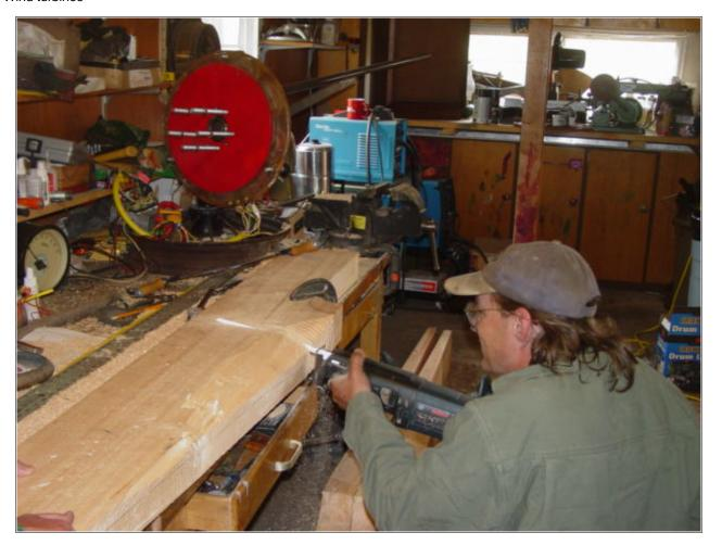
Pictured above Matt's curfing the blades with a sawzall. This goes very quickly - we only do it near the root. Once a lot of slots get cut, we knock out the chips with a chizel.
