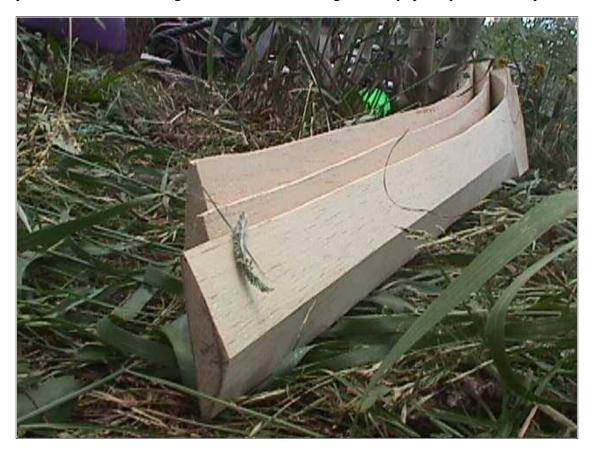
To rough out the airfoil, First we plane (I use a power planer) the back side of the prop down so it's to the right thickness. (3/8" at the tips tapered to full board thickness at the root) Then I draw a line, 1/3 of the way back from the front (leading edge) of the prop, and use the draw knife (and power planer) to basicly carve it into a triangle. From here it's quick to use the drawknife and the power planer to make a nice looking airfoil.
