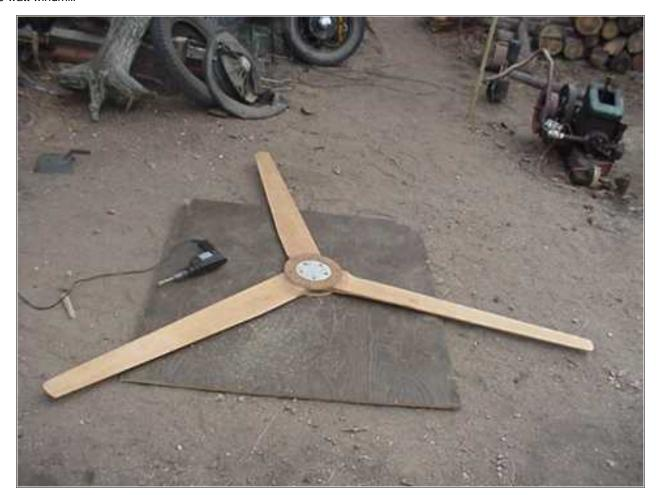
We actually had to make two props for this, since we accidently dropped the machine in our first attempt to raise it! Click here to read about that failure! The first prop we made out of the very best, vertical grain knot free fur. The second prop we made out of some fairly clean Lodgepole pine we had on hand. Both worked well, the 2nd prop actually runs somewhat quieter due to reduced thickness. Otherwise, they are about the same and this page will document only the creation of the 1st one!
