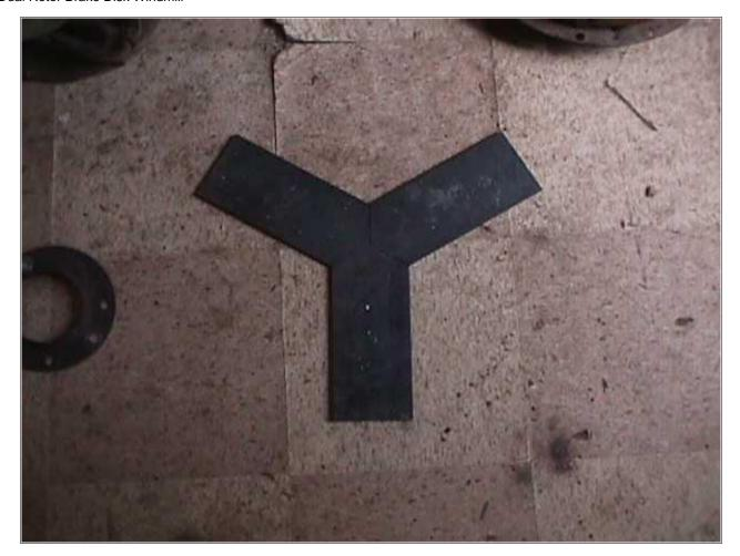
Above you can see how those go together. After this we drilled holes in the center to bolt it down, and a large 1.75" dia hole in the center for the wheel spindle to pass through. We also need to drill holes out at the ends to accept allthread so we can mount the stator to it.
