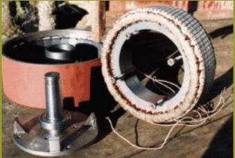
Here are parts of the alternator. The magnet rotor (top left) is cast from iron. It runs on the main shaft. The blades are bolted to the face this rotor. Inside the rotor are ferrite permanent magnets. The magnets move past the laminated core of the stator which contains stationary coils of copper wire. On the right you can see the stator being wound.
