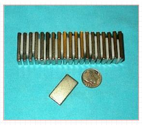
More Neodymium magnets for those on a budget. They make nice alternators as shown in the section "Alt from scratch"
