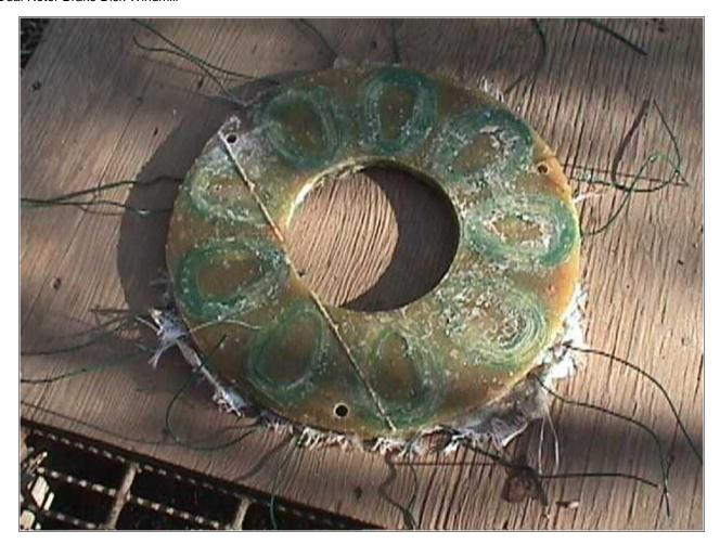
After about 2 hours we opened the mold and took the stator out.
