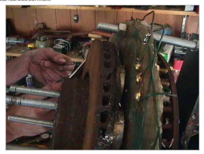
We soldered all the connections on the stator and made 6 lugs (2 for each phase) from brass screws and brass nuts. It can get tedious stripping all the ends of the magnet wire, a good way is to burn the insulation off with a propane torch, and then sand it lightly.
