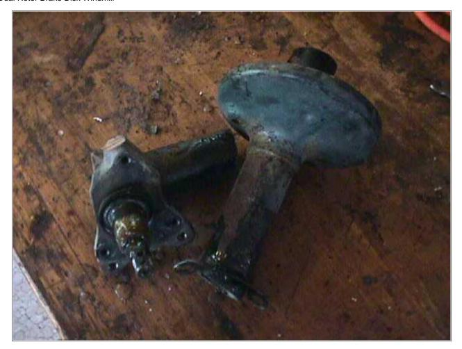
To make the furling tail assembly, I cut the strut about 6" from the wheel spindle. We want the spindle (and therefor the alternator and the prop) to be offset from the tower about 5" to the side.
