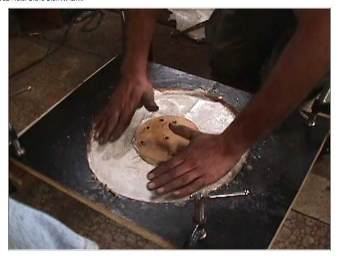
Pictured above is the mold we made for the stator, and we're putting some fiberglass fabric in the bottom to strengthen it.
