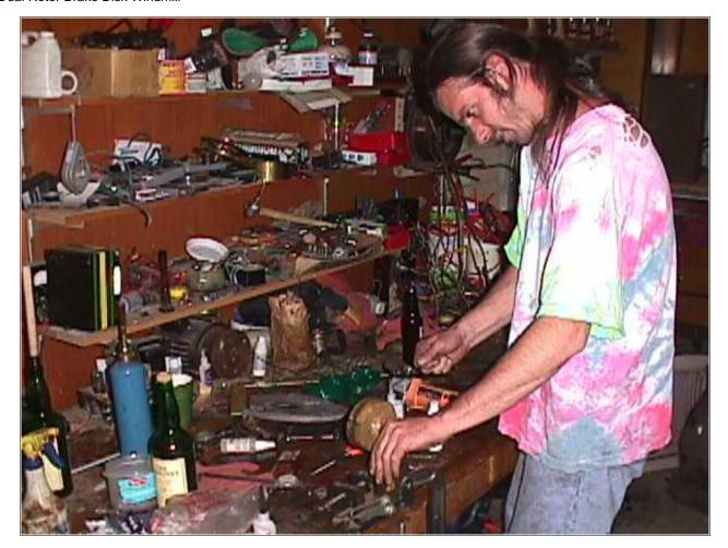
Pictured above Dave is winding up some coils. Just like my last one, each coil occupies the space of about 1 and 1/3 magnets (so 3 coils take up space occupied by 4 magnets, so there are 9 coils in the stator). Its 3 phase, so each phase consists of 3 coils in series. The coils are made up of 65 windings of AWG 14 wire.
