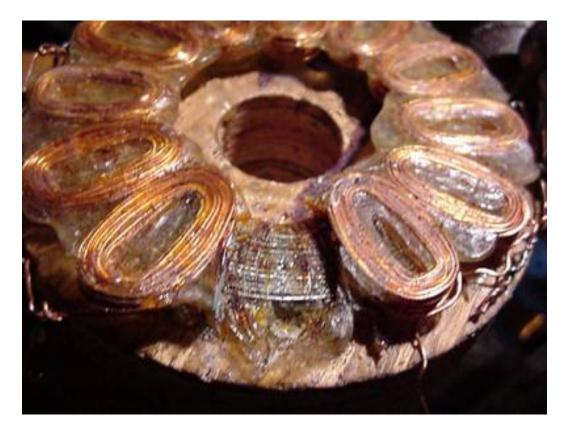
Removing the bad coil was much like doing dentistry with a hacksaw and chisel...OUCH!
