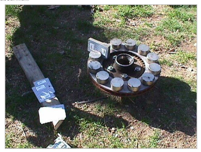
The magnets lay down on the brake disk such that each one has the opposite pole facing up as the one next to it. Alternating North and South poles all around the disk. I push the magnets all the way out to the lip I cut and space them approximately by eye. Then I use shims (playing cards) and go 'round the circle so they are perfectly spaced. The space between the magnets here is about 1/2 inch (or exactly the thickness of 49 playing cards).
