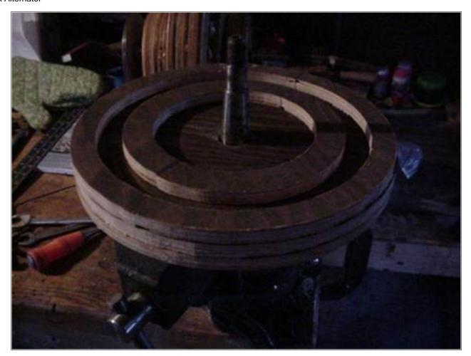
Pictured above is the beginning of the plywood stator. It is made out of laminated plywood discs. The total thickness is 1.5". The top layer, which is 1/2" thick, has a slot 1" wide at about 10" diameter so that steel laminates can be epoxied in. Over that will be the coils. (you'll see this later in the page!)
