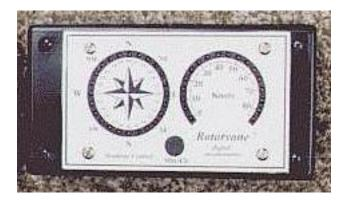
Web-based weather servers and other computers can read the wind data directly from its serial port. Its serial port can be connected to a modem, allowing remote wind monitoring via a dialup line.
