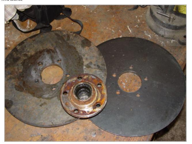
Above we have the machined rotors and the wheel hub they'll fit onto. There is the large hole in the middle, 5 1/2" dia holes that fit the studs, and then 3 holes (smaller) which are tapped for 1/2" - 13 bolts. These last 3 holes are used for jacking screws which we need to safely put the magnetic rotors together and take them apart. The attraction of these two disks is VERY powerful, wthout jacking screws it would be impossible.
