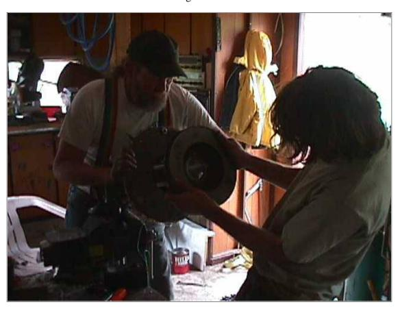
Now we need to prepare for the 2nd magnet rotor. We have no magnets on the rotor yet, so it's somewhat safer to handle. I take the rotor, holding it backwards (so the magnetic force of the back rotor doesn't grab it too hard), and see if the 5 holes in it line up nicely with the half in studs. Usually it doesn't, because the studs bend around a bit when we tighen them to the wheel hub! But this test gives us an idea how far off they are.
