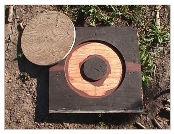
Pictured above is the finished mold. The dark purple spots are caulk we used to fill gaps and cracks between wood... this just helps the casting come out more easily. Before using the mold, we need to put some kind of release agent in there. Auto polish wax works great... we didn't have any so we used axle grease! Lard, butter... I'm sure lots of things would work fine!
