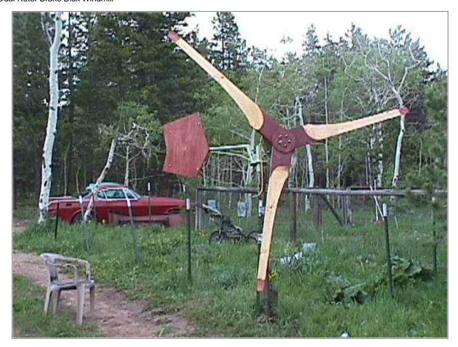
Thats pretty much where we wound up at the end of day 3! We used wood stain on the hub and tips of the prop, and on the tail. The rest is good old Avacado green epoxy appliance enamel just like on my last machine. At this point we need to make adjustments in the airgap, get some wobble out of the magnet rotor on the front, balance the blades and test it!
