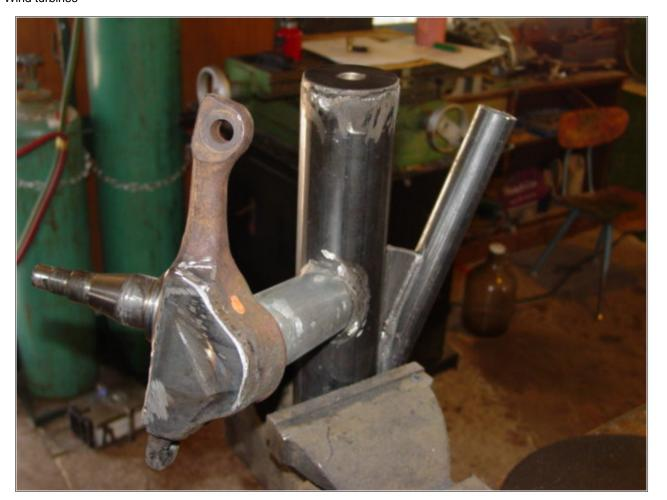
Here we have the yaw bearing, the alternator spindle, and the tail pivot all welded together. The top piece on the yaw bearing is actually the center of one of the magnet rotors which was cutout with a hole saw, it made a nice heavy washer to hold her on top of the tower. The spindle on which the alternator will turn is tipped up a couple deg to help keep the blade tips out of the tower. It adds a bit of insurance and I think it looks kind of sporty that way!
