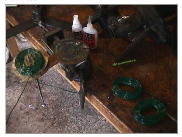
Pictured above is the glue, the coil winder with the lid off showing a coil... and a few coils I wound. Once all 9 coils are wound we're almost ready to build the stator! First we have to make a mold.
