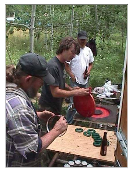
Pictured above we are wiping axle grease all over the mold to assure things will come out easily in the end.
