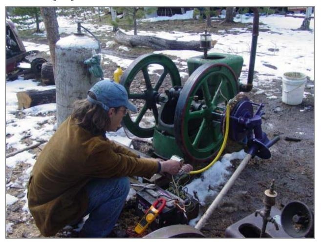
Above Im trying to get some data on one of the brake disk alternators which are intended to run with a 10' diameter prop. <u>Click Here</u> to see a page about identical wind turbines with identical alternators and their construction.
