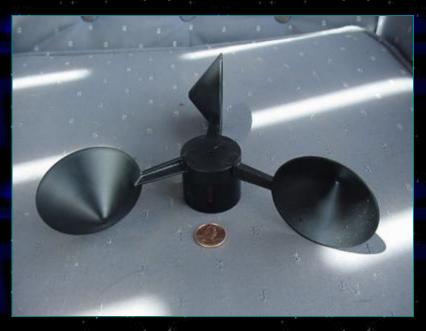
unassembled, and the cups simply press fit very firmly into the hub -- no glue is needed. In both of the anemometers we built with these cups, no balancing was needed. There is a 3/32 inch diameter reinforced hole in the exact center of the hub to make fitting your own shaft, bearing, or surplus gadget to the hub fast and easy.
