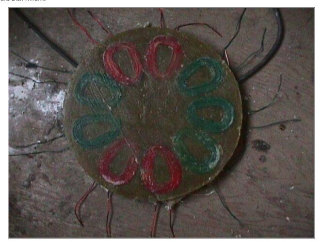
After a couple hours I opened the mold and the stator is pictured above.
