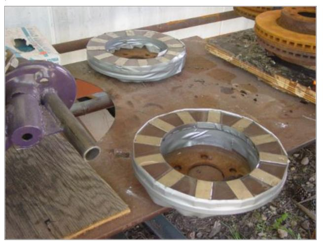
We used Polyester fiberglass resin for casting both the stator, and the magnet rotors. Here the resin is setting up, once hard the magnet rotors will be finished.
