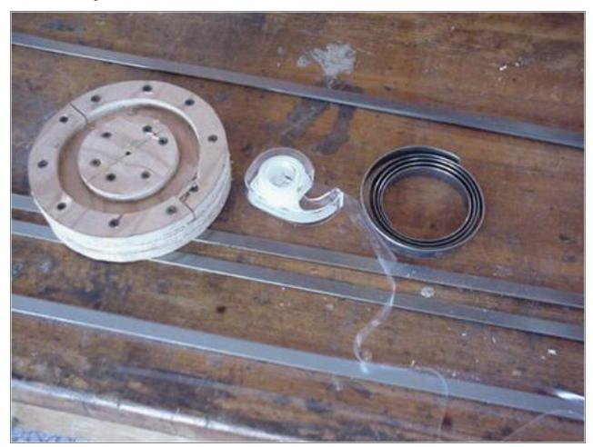
Show above is the plywood stator, glued, and screwed together. You can clearly see the cavity into which the laminates will be glued in. The laminates are made up of 1/2" wide strips of 20 gage cold rolled steel sheet metal. The strips I used are 4' long, and before installing them, I covered 1 side of each strip with tape so that each piece would be insulated from the one beside it! This is very important to reduce eddy currents.
