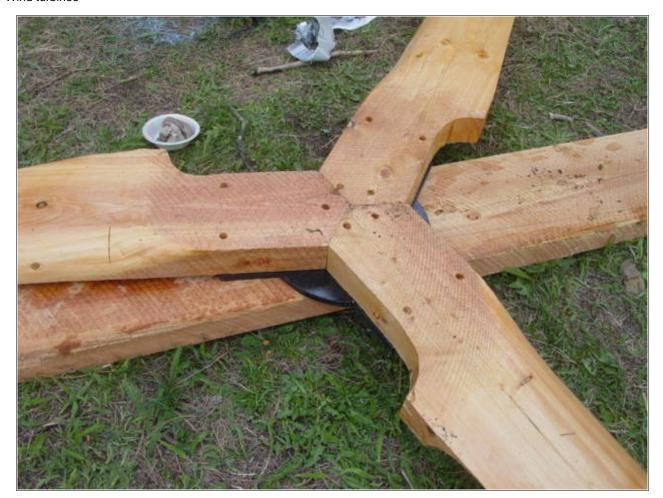
All the holes came out nice and square and on location. In this picture we have the front hub screwed down and were preparing to put the back hub on. It all fit quite well. We painted the hub disks, and finished the blades in linseed oil before assembly.
