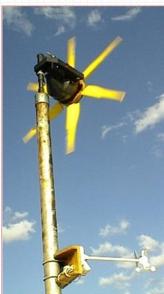
The downwind turbine, a very small but quite efficient little unit. This one was a bit more complicated to build but it features the star/delta controller ( check the link on downwind turbine for more detail)
