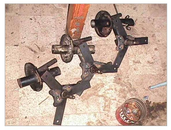
Pictured above we've welded the stator brackets to the main chassis of the wind turbine. This is a good time to prepare the stator for mounting.
