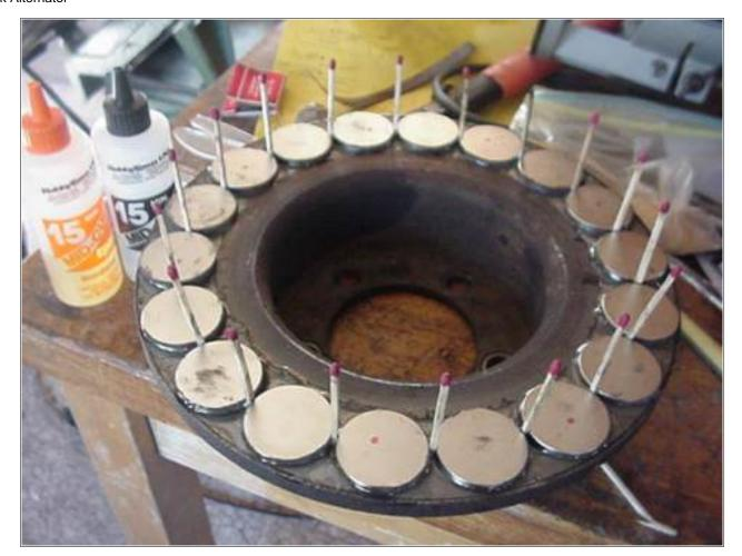
While I had the glue out, I glued the magnets into the brake disk at the same time. Once the glue set up partially, I removed the matchstick spacers.
