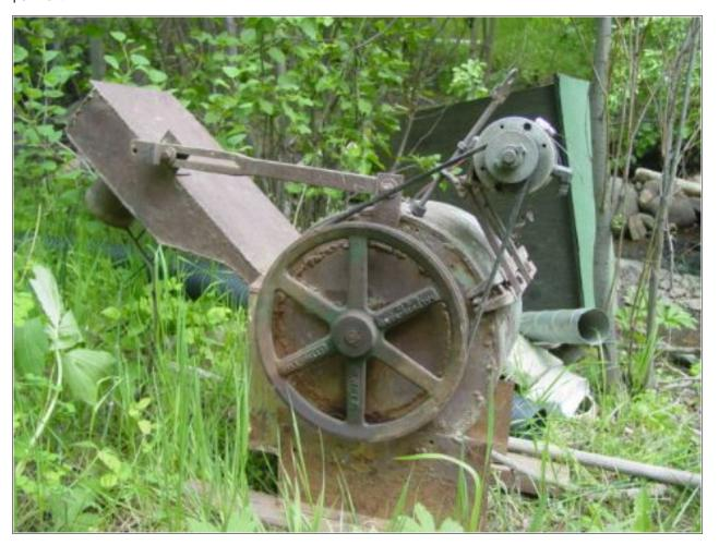
This is Scott's old machine, which ran for 2 years even through the winter. Again, it was good for about 1 amp (12 watts) or so. It's a squirrel cage blower, belted up to an Ametek computer tape drive motor. To get an amp from it, the belt tension was very critical and required frequent adjustment. It was a good machine though! Hopefully what were doing here will be an improvement...
