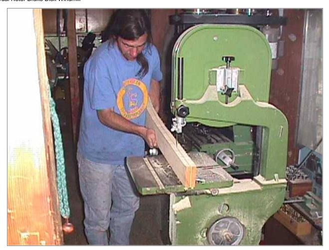
Since the blades get very thin (in this case about 3/8") at the tips, it saves time to remove some of the thickness of the board with the bandsaw.
