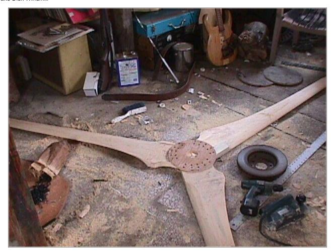
The blades are sandwiched between two plywood disks and held together with a ton of screws. In the past I've used glue here, but I opted not to this time thinking that the screws, along with the tight squeezing that happens when the prop is bolted on would be good enough. This way if I ever need to replace one blade it will be easy.
