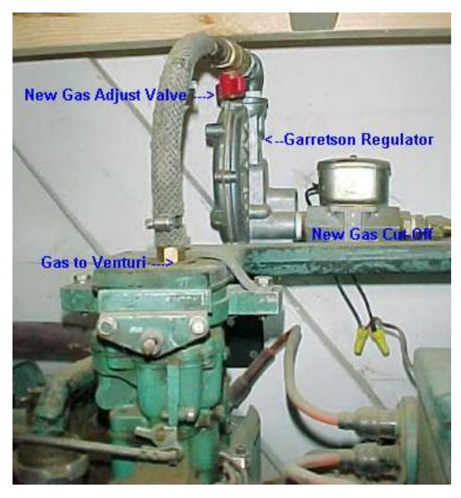
Examine the above photo carefully, and identify the new parts for the conversion!
