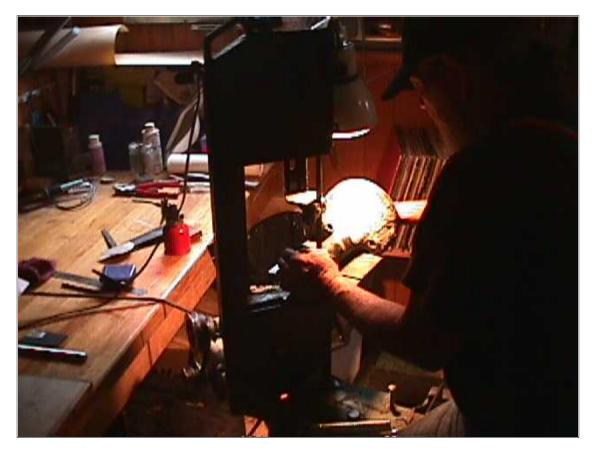
Tom is cutting pieces on the saw. It's nice to get a list of all the parts you need to cut and get it over with in one shot. Here Tom is cutting a 5' piece of 3/4" pipe, 5 pieces of 1/2"-13 allthread 10" long, 3 pieces of
