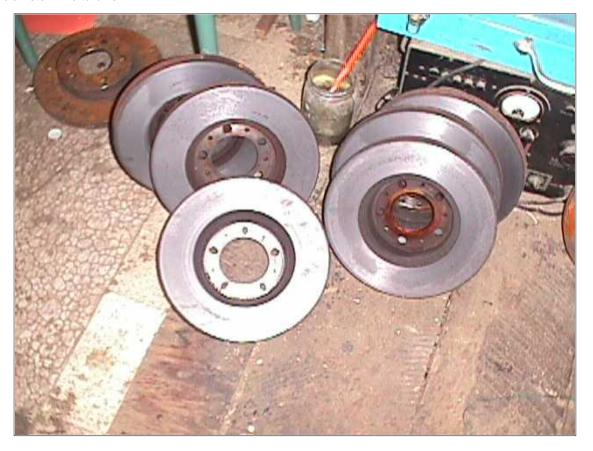
Above is shown the brake rotors after being turned. You can see that the hole in the ones on the left is slightly larger than those on the right. After machining them, we clean them carefully with paint thinner or gasoline so that we can glue the magnets on later.
