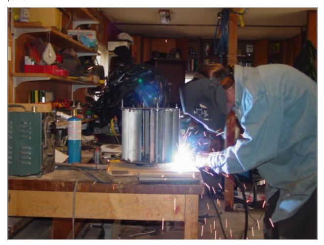
Here the runner is getting welded up. It's important to note... the vanes are made of galvanized steel conduit. We had to grind all the galvanization (Zinc) off the edges before welding this... welding galvanized metal produces toxic gas, so we try to be careful about this.
