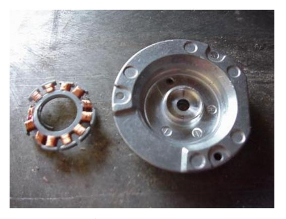
**Coils removed from Motor**
