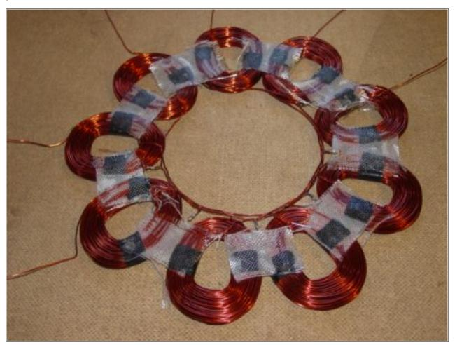
We made the connections on the stator and it's ready for casting. Each coil has 125 windings of #17 wire. Each phase has 3 coils in series, and we'll be bringing out 6 leads, so that we can choose between the Star, or Delta configuration.
