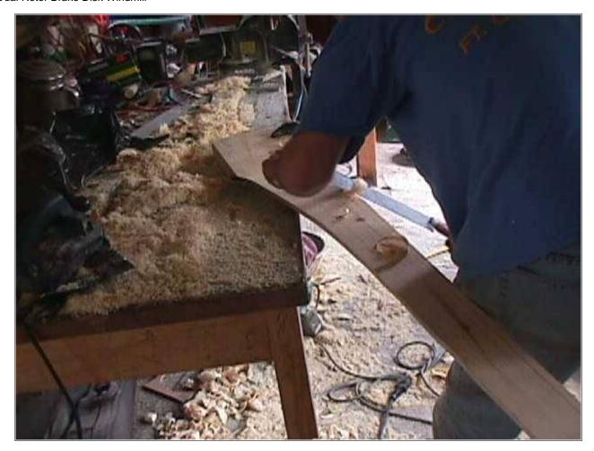
Here we are roughing out the back side of the blade (making an airfoil) with the draw knife.
