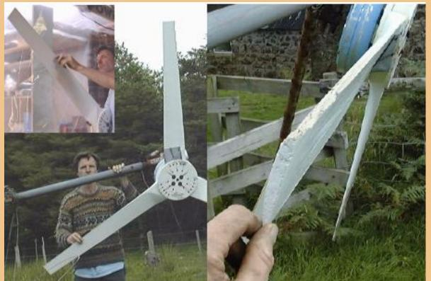
It looks as if I forgot to put epoxy resin on the blade edges! Otherwise it works fine. The grey patch on the topmost blade is a piece of lead flashing (used in roofing) screwed on as a balance weight. Normally a smaller weight will do!
