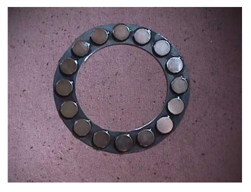
Magnets mounted on steel ring
