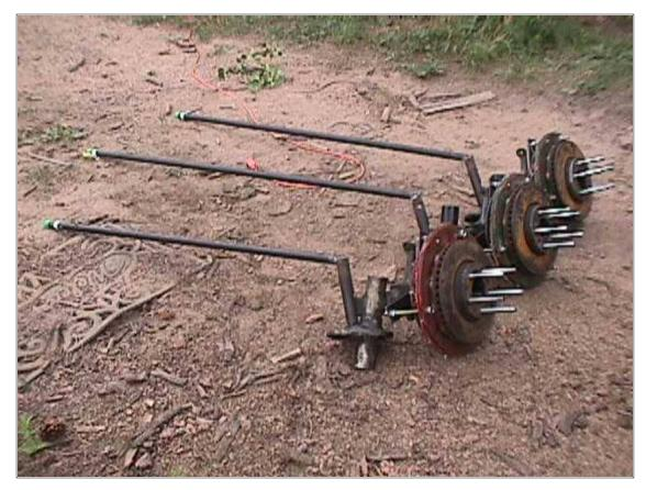
Pictured above we have 3 machines very nearly finished except for tails, paint, and props. The tails we'll put on here by welding brackets of 1" wide, 1/8" thick steel bar stock near the end of the tail boom. Again, the tail boom is 3/4" pipe, 5' long. The tail itself will be made of 3/8" plywood, and will be about 5 square feet in area.
