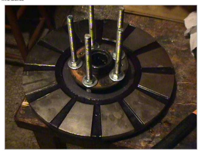
Pictured above the back magnet rotor is mounted to the wheel hub. I like to keep the back rotor towards the rear as much as possible, this will keep the hardware that mounts the stator shorter so that it's stronger and more compact. The rotors are held to the hub with 1/2 - 13 allthread and nuts.
