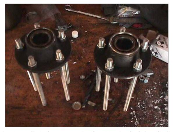
This was shown in an earlier drawing on page one. Once the studs have been knocked out with a hammer, we replace them with 10" long pieces of 1/2"-13 allthread. The new 10" studs are held to the wheel hub with a nut on each side. We need to leave about 1" of thread sticking out past the nut on the back side so there will be room for
