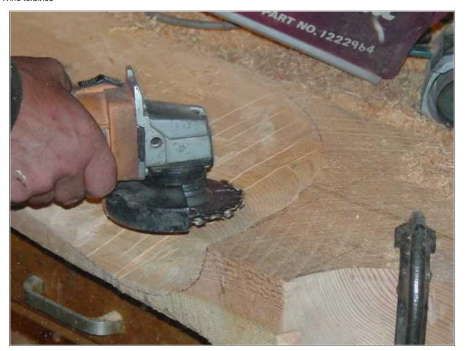
I think it's called a 'lancelot'... a wicked tool, possibly the most dangerous power tool I've ever used. Once used to it though, it does a nice job of removing wood quickly and precisely. It's useful down at the root of the blade.
