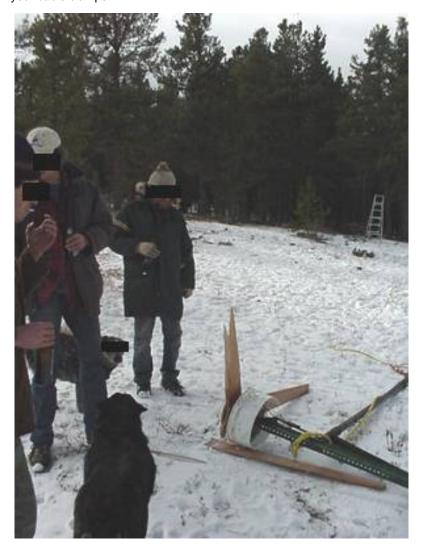
Fortunately, there was no damage to the alternator itself. The cowling, made from a plastic bucket and wooden spacers, saved the alternator's stator coils! Ward's nice rotor, lovingly crafted with flawless, knotless and very expensive Douglas Fir and finished with about \$40 worth of cyanoacrylate, is toast. Though one blade did survive!
