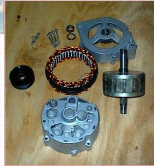
One of the original alternator modifications. This one had a rewound stator and the modified rotor using Neo' magnets.
