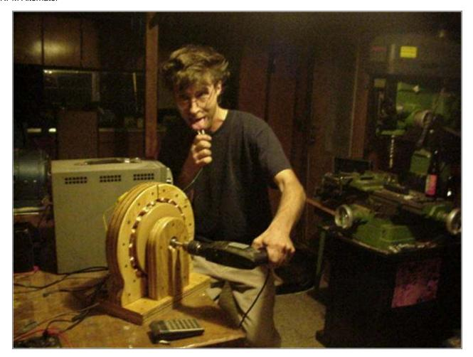
All the coils on each half of the stator are wired together in series. At that point, each half can be hooked in either series or parallel to most appropriately match the load with the alternator. Above is pictured the good old Taste Test, a sure fire way to test any battery, or generator, as long as it stays below about 10 volts! (otherwise it hurts--don't try this at home!)
