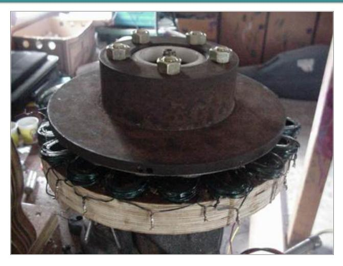
The completed unit. It's already been attached to a homebrew wind generator with an 8-foot diameter, 3-bladed rotor--and is up and flying! See it HERE! We've already seen peaks of over 60 amps into a 12 volt battery bank, and it survived 60-mph winds last week. Steady output of 30 amps in 28 mph winds, and reaches charging voltage at around 12 mph.
