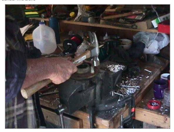
The wheel hub still has the original studs which used to hold the tire on the car. These are simply a press fit, and they are quickly knocked out with a hammer.
