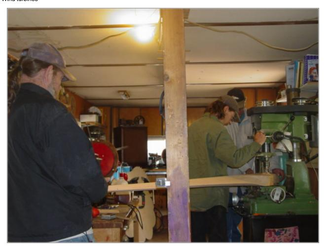
A 15' blade set is much too large to assemble in my small shop. We had to layout each side of the hub seperately, and drill those out. Once the hub parts (basicly disks of 3/4" plywood) were drilled out, we marked where the holes would be in the blades, and drilled out each blade individually.
