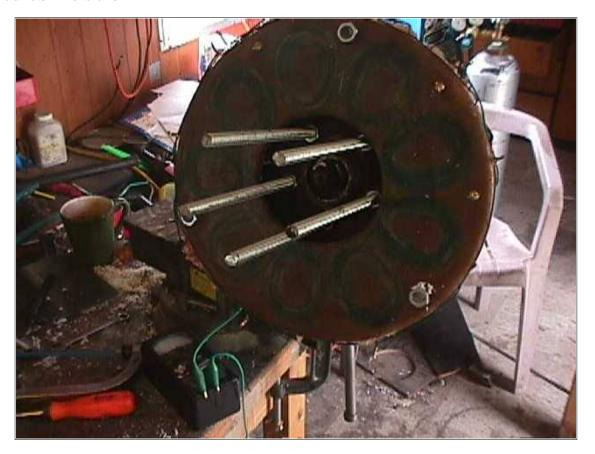
At this point we have the stator wired, soldered, and you can see the 3 brass screws we used for terminals. I like to take some epoxy at this point (once all the connections are tested) and glue the wires down around the edge of the stator to protect them, and keep them from vibrating. DanF is building a cowling around his stator to keep the wind from vibrating the solder connections.
