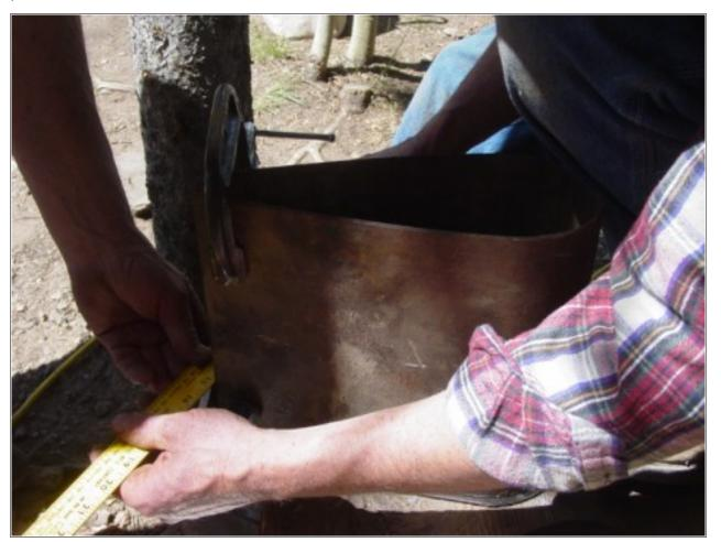
The nozzel will be the same width (10") as the runner, and it's about 1" wide where the water exits. This gives about the same area at the end of the nozzel as the 4" pipe that feeds it... slightly less. Pictured above we're bending the sheet metal which makes it up.
