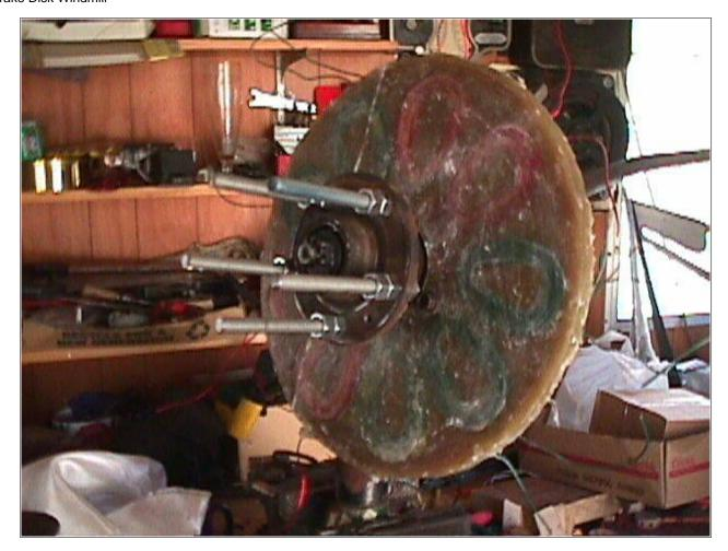
Pictured above is the stator bolted onto the machine. I've also got the wheel hub on here. You can see how the studs (where the lugnuts used to go) have been replaced by longer (7 inch long) pieces of 1/2 inch allthread. The studs were pressed in, and are easily knocked out with a hammer. The allthread is held on with nuts on each side, and then another nut is used on each one to hold the magnet rotor out the proper distance so that the magnets run very near (about 1/8 inch) the stator.
