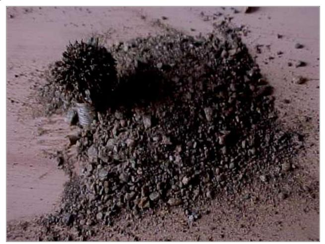
I dragged a magnet around in the dirt of my driveway, so that it would attract the magnetite sand. Pictured above you can see the pile I used, with a stack of magnets demonstrating its magnetic properties.
