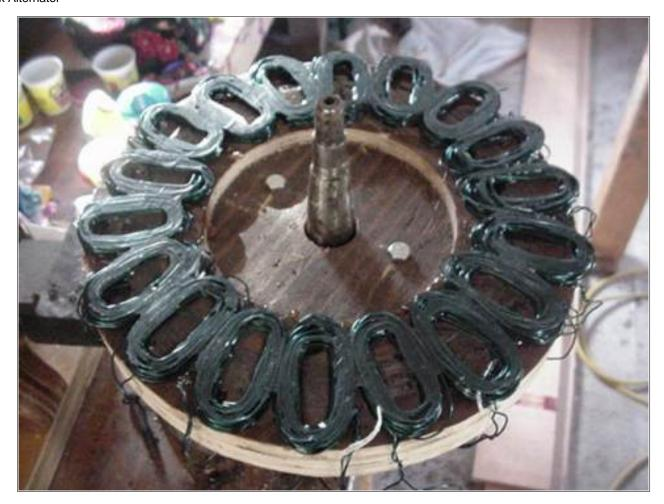
Above is pictured the stator, mostly complete, with the coils smashed down tightly and glued well. At this point, I coated the assembly (plywood front and back) with epoxy to weather proof it as best I could. I divided the coils in half, hooking 2 sets of 9 coils together in series and figured I would decide later whether to hook the two halves in series or parallel - this was not decided untill a prop was made and I actually got to test it in known windspeeds.
