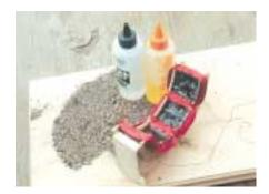
We separated this somewhat magnetic sand into a pile, sifted it through a window screen, and sorted that with the magnet one more time. The remaining black sand sticking to the magnet was nearly pure magnetite. A quick test of any local dirt pile with a neodymium magnet should reveal whether your sand contains magnetite. If not, try dragging the magnet along the sandy bottom of a local river. Any deposits of black sand on the river bottom are most likely nearly pure magnetite.
