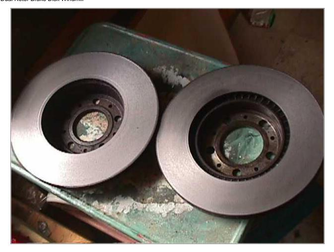
This is how the brake rotors look after cutting them down to make a lip on the outside which holds things together. I don't think this step is necessary - but it's easy and provides some insurance against magnets flying loose. It also makes a nice clean flat surface to put the magnets down onto.
