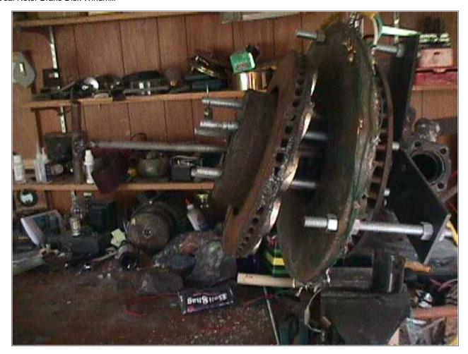
Here is a picture of the wheel puller in action. It doesn't pull it quite straight, but it does a good enough job to make it very easy to pull the rotor off by hand once it's a few inches back.
