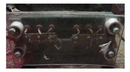
home built diode bridge--note the insulated standoffs so the diodes don't ground to the case.
