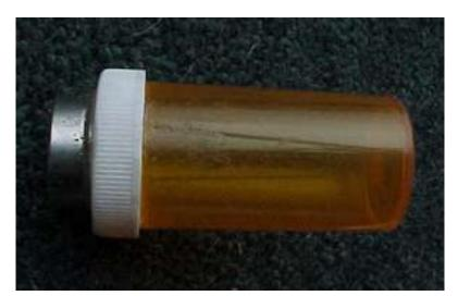
Float with magnet glued on top
