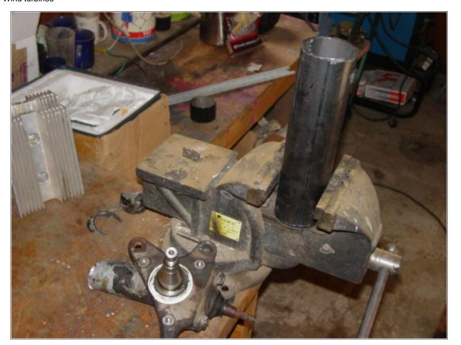
Pictured above is the wheel spindle with about 7" of the strut towers tubing attached. Instead of using the strut tower's tubing for the yaw bearing like we did on past machines, this time we'll weld the spindle to a stronger piece of 2.5" diameter pipe.
