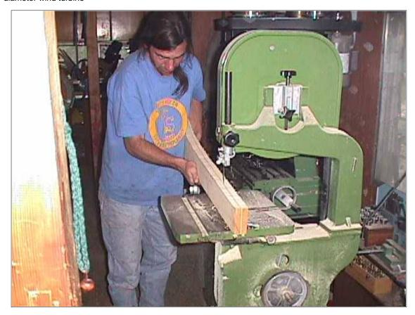
As per the drawing above, the tips of the blades are only 3/8" thick, and the root is full thickness. So quite a bit of material needs to be removed. Pictured above we are cutting off this extra wood on the bandsaw. We leave a bit of extra, just in case we make a mistake with the saw, it gets tricky ripping through the thickest part of a board this way, it's best to leave some room for error.
