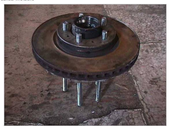
This shows how the back rotor fits over the wheel hub. Had we not turned out the center hole on a bit larger, the hub could not have fit through like this as the rotor was never designed to fit on in this way. Now we only need to tighten 5 nuts over these studs and locktight them.
