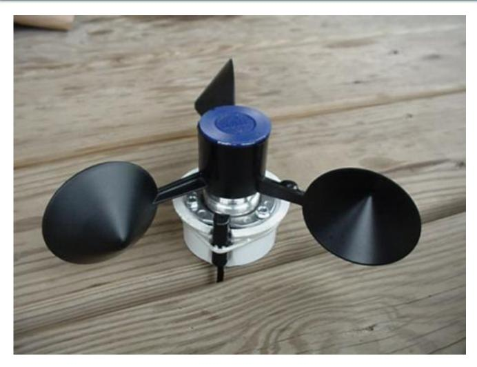
The completed anemometer cup and sensor assembly.
