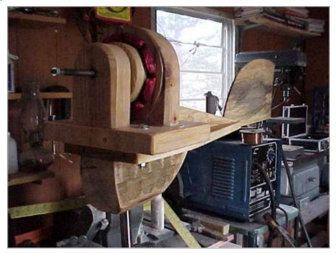
To stay with the "style" of the project I decided to build the whole windmill out of wood, it's a fairly simple design and should be self explanatory. It's glued and pinned, with wooden dowels, no bolts are used except to bolt the alternator on it. I cheated there.
