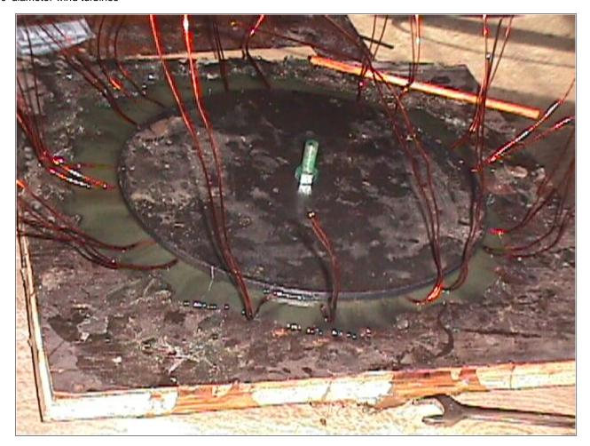
A small improvement to the stator mould. Here we have Scott's stator setting up. For the lid of the mould we used a 14" diameter steel disk and bolted it down tightly with a 1/2" bolt/nut. This made the stator come out very nice and thin - it was much nicer than using clamps or screws like we have before.
