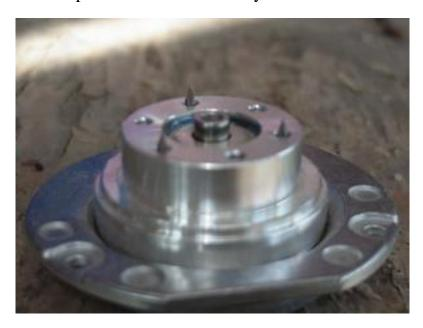
Nails in motor for marking hub holes.
