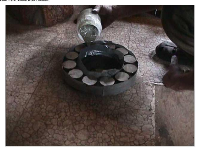
Here we are pouring resin (mixed with talcom powder) into the magnet rotor. Well have to make 2 magnet rotors, but for now we're just doing one. It is possible the alternator will work OK with only one magnet rotor and the other rotor simply serving to conduct the field of these magnets (like laminates except itll be rotating) - so were not doing the 2nd rotor untill we test the alternator. We may even decide to use different magnets on the 2nd one.
