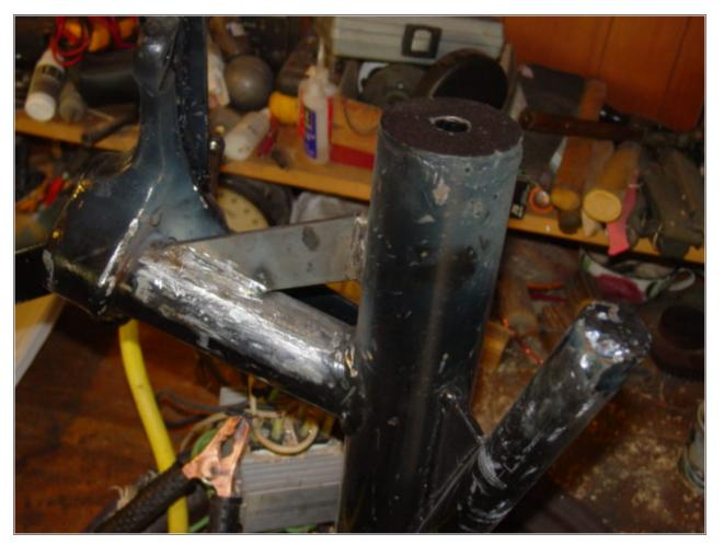
I added a gusset to the tube that offsets the alternator, and filled the tail pivot with 1/8" diameter stainless steel rods, and welded it over. This should make it a bit stronger. I had some concerns about the tail pivot cracking.
