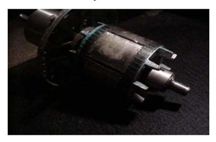
Armature converted with permanent magnets
