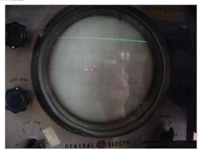
See above the nice, flat DC output after a capacitor is hooked up between Pos and Neg outputs.
