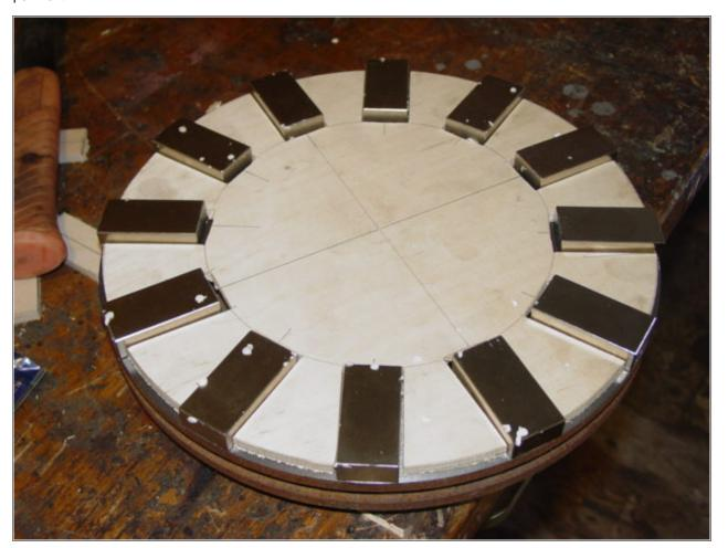
Pictured above we have the magnets positioned, and the template in place. The magnets are 1" X 2" X 1/2" thick, there are 12 on each rotor. This part of the machine is almost identical to the alternator in <a href="Hugh Piggott's Axial Flux Wind Turbine plans">Hugh Piggott's Axial Flux Wind Turbine plans</a>. The magnets are available <a href="HERE">HERE</a>.
