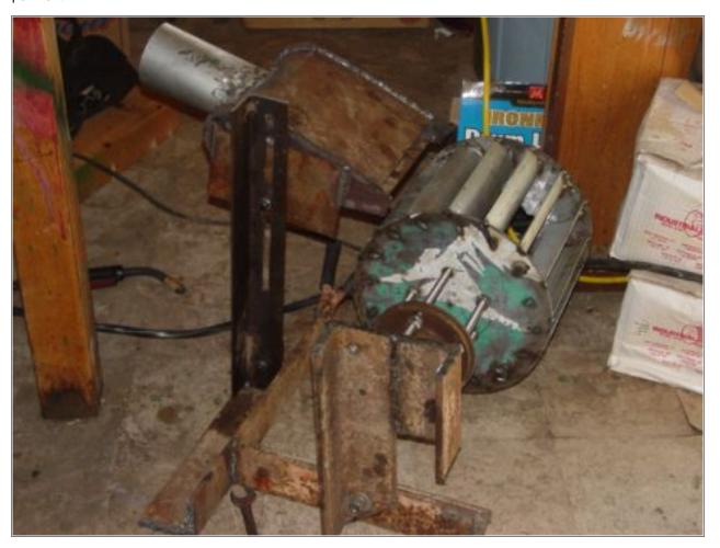
Pictured above it's starting to take shape. We've mounted the runner to the hub, and basicly assembled everyting except for the alternator. Everything on this is adjustable. We can move the nozzel forward, back, up, and down. The runner (and the alternator) can be moved back, and fourth.
