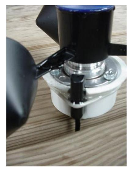
Completed anemometer hub assembly, mounted in PVC reducer, with sensor attached.
