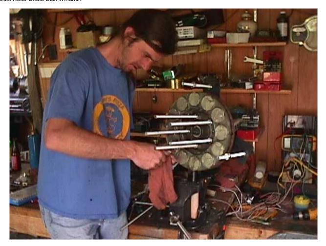
Here were putting allthread and nuts into the stator bracket to hold the stator on. The allthread is 1/2" diameter with 13 threads per inch.
