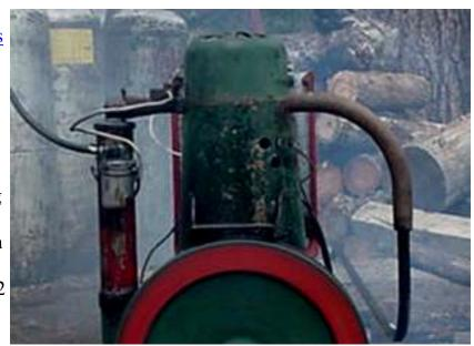
volts. Mine runs well on gasoline, but seems to prefer kerosene, or diesel. Its good for about 25 amps at 12 volts, and consumes a little over 1 pint of fuel per hour(a little less with kerosene, a little more with gasoline). Surprisingly, it seems to run best of all on citronella tiki lamp oil, which is probably mostly kerosene. And we've had
