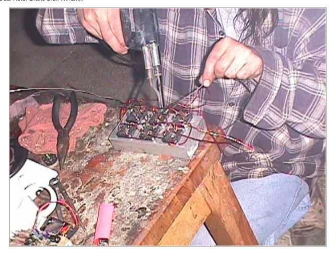
Here Dave is soldering up 6 bridge rectifiers we'll need in order to convert the 3 phase AC current into DC current useful for charging batteries.
