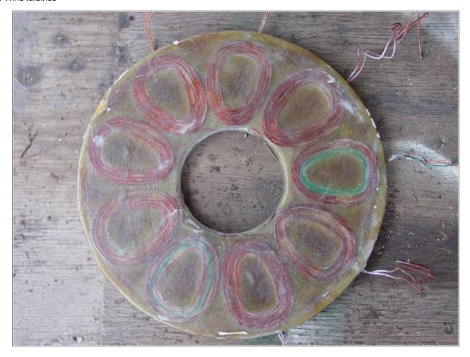
Once the coils are all wired up, we put them in the mould and cast them in polyester resin with fiberglass mat to strengthen it. Here we have a nice 24 volt stator fresh out of the mould.
