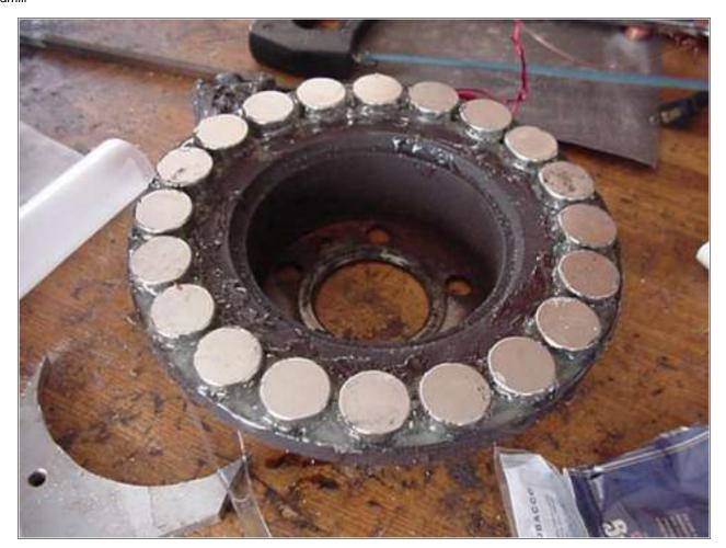
Above you can see the brake rotor with magnets installed. There are 20 magnets in this one, each one is 1.25" diameter X 0.5" thick. Its important that they be perfectly spaced. I cut a shallow slot (about 1/8" thick) in the brake rotor, with inner diameter of exactly 9.25" and outer 10.5" which holds the magnets in place. I spaced the magnets out perfectly, and epoxied them in place. This finished assembly is the "armature".
