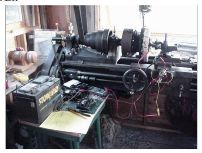
Pictured above is the "test rig." It's somewhat limited by the motor on my lathe - the max speed I could test it at was 500 rpm, and even at that speed it loads up the motor and slows it down. The problem is that my lathe only has a 1/2 hp motor on it. The reason for this is that I run my whole shop off my batteries and a "cheap Chinese" inverter! Someday I'll upgrade to a 1 hp motor, which my inverter should barely run...but for now my tests are limited.
