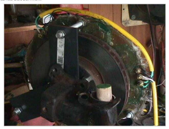
While Dave was planing on the blades I made up a cable with lugs on it and wired the alternator in Delta. For more details on Star, or Delta wiring and 3 phase alternators, checkout Ed's 3 phase basics <a href="here.">here.</a>
