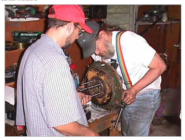
In the picture above we are hand turning the alternator and testing for output.
