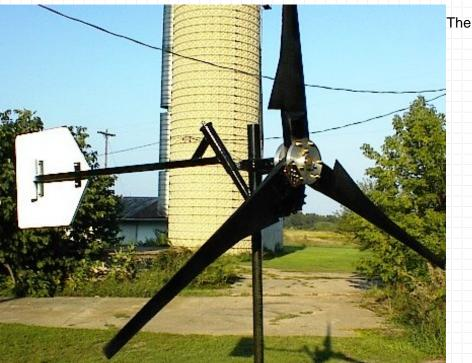
original 6 ft turbine with a car alternator and chain drive. It was changed to the axial Flux type alternator and ended up being much more efficient and powerful. The chain drive was quite noisey because of the cogging in the modified alternator. It was in service for about 2 years and is now down for maintenance. Actually it will be refitted with a new alternator using the new magnets and the blades refurbished.
