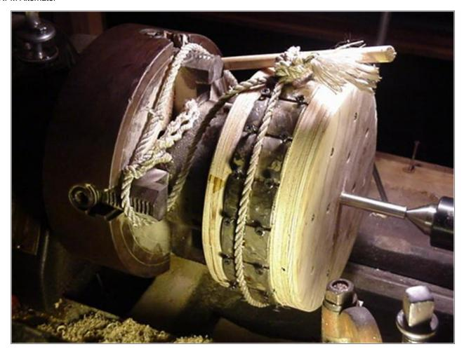
Once all the magnets were pressed in place, properly spaced with screws, I glued them in with epoxy. As a clamp, I simply tied a rope around the magnets and tightened it with a stick through the knot. When the glue started to set up hard, I removed the screws and applied a new coat of glue over the entire surface of the alternator. This not only aids in holding down the magnets, but it will protect the alternator from moisture.
