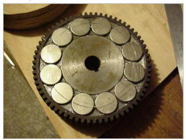
I cut a slot in the gear 1" wide, and about 1/8" deep to hold the magnets in. The magnets must be evenly spaced around the circle, and once they were, I glued them in with epoxy. This is very similar to the Volvo disk brake alternator I made - so check that page out for more detail. The polarity of the magnets around the circle alternates, so each magnet has the opposite pole up as its neighbor.
