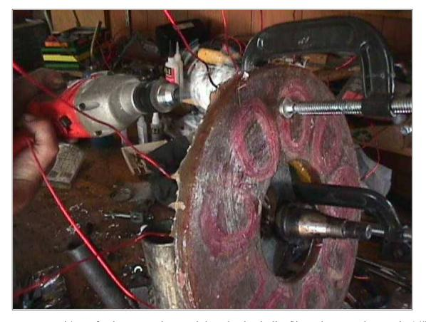
We line the stator up so it's perfectly centered around the wheel spindle. Since the stator is exactly 14" diameter, and each leg of the stator bracket is 7" long, the edges of the stator should line up perfectly with the edges of the stator bracket. We've drilled 1/2" holes in the stator bracket for mounting. We need to position the stator so that
