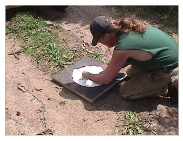
We need some fiberglass in the stator for strength. Pictured above DanF is cutting out 2 rings of fiberglass fabric exactly the size of the stator, 14" diameter with a 5" hole in the middle. We'll have one of these on each side of the coils for reinforcement.
