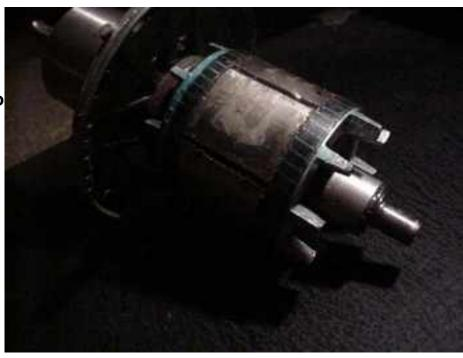
to the bike, I was able to generate 5 amps(60 watts) in a leisurely way, and if I pedaled as fast as I could, I'd get about 10 amps(120 watts). This seems to be in line with claims we've seen for other peoples plans, although it seems clear that with a higher gear ratio, one could generate significantly more with this alternator.
