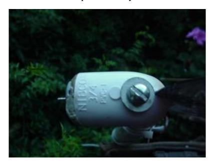
Top view showing yaw bearing bolt
