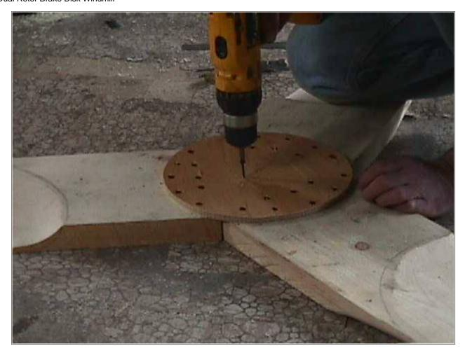
Once the blades were carved and sanded fairly smooth, we put them together - measuring from tip to tip to make sure the distance between tips is equal. Then we used 10 inch diameter plywood disks, one half inch thick, and screwed one on each side of the blades with a ton of wood screws to hold them together.
