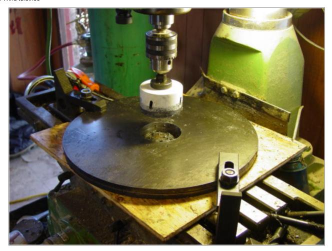
After it's layed out, I piled up both disks and drilled them at the same time. The center is easy to cutout with a holesaw, the diamter is such that the hub fits through the hole, I believe it was 2.75".
