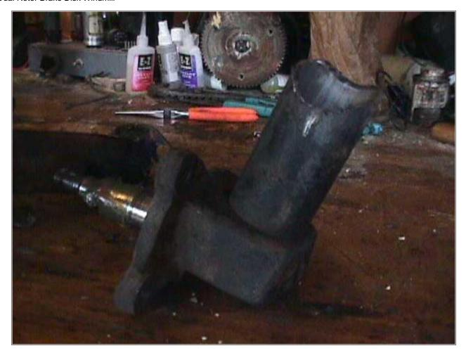
I ground it out so its a good fit for welding. It will be welded on at an angle to provide more contact between the two pieces making the joint stronger. I also like to weld it on so that the spindle (and therefor the alternator and the prop) is pointed up about 2 deg to help keep the tips of the blade away from the tower.
