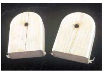
forced it through the holes. This gave a good tight fit, hardened the wood, and made a layer of carbon on the inside for better lubrication. We drilled a small hole in the top of each pillow block, down into the shaft hole, so the bearings can be greased.
