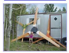
We did it *completely* from scratch this time--cutting the tree, hauling it to the sawmill, milling it, and carving the blades! The blades are for a 16 foot dia turbine that's going in at MattB's house. Click the photo to check out the web page about the project.
