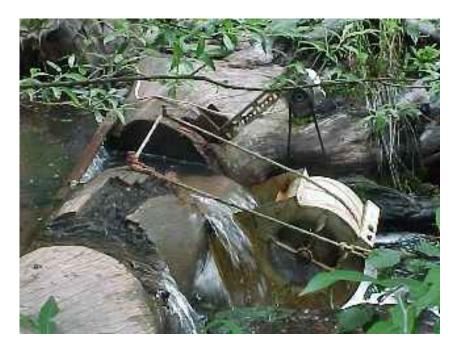
A while back, one of our neighbors constructed a water wheel generator using a squirrel cage fan, belt, pulley and surplus tape drive motor that produced a steady 1-2 amps of power, 24 hours a day. He used a natural dam (a log that fell across the creek years ago) to get the fall and to mount the generator on. Click here for more information on this clever water wheel.
