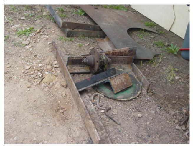
We started with scraps of sheet metal and angle iron. The disks for the runner were made from the base of a dead Onan Generator. The alternator was built from two 11" diameter brake rotors (we think they are off a Dodge but not sure), and the spindle/wheel hub also... probably from a Dodge, but were not sure because it was salvaged off other homemade equipment.
