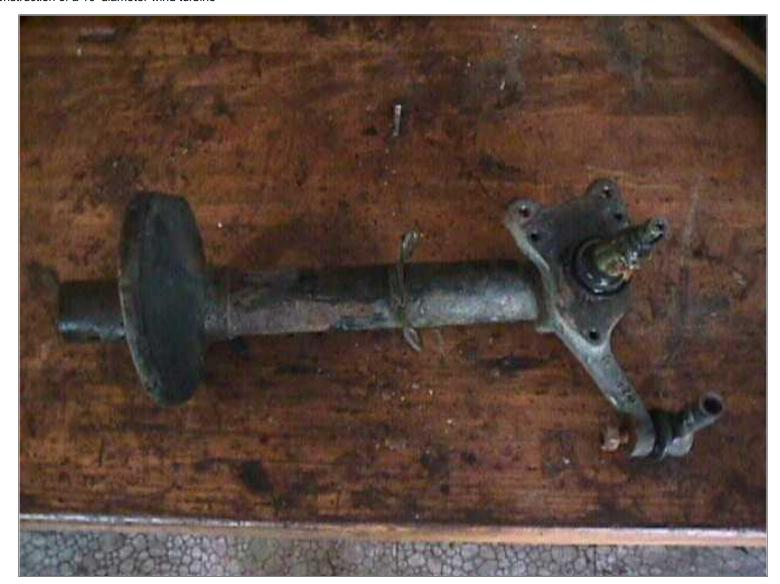
Above we can see the strut assembly mostly stripped of it's extra parts. The picture below will show how we need to cut this up and weld it back together to make the furling system work.
