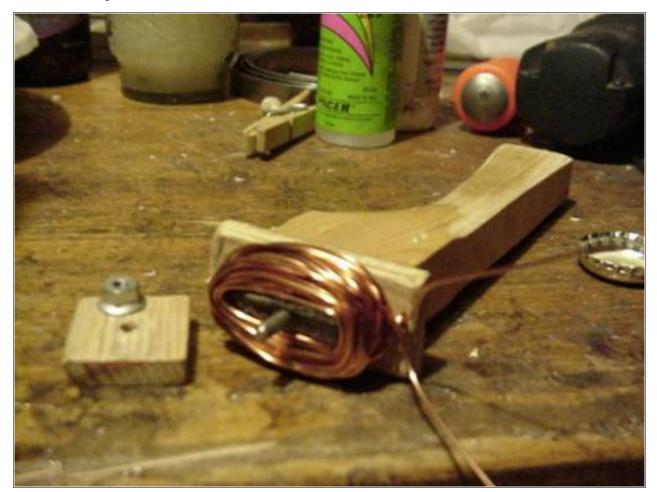
Above is shown the same coil winder with a finished coil on it. Each coil is made up of 40 turns of AWG 18 magnet wire. Once the coils are finished, I twisted the ends tightly together before removing them from the winder.
