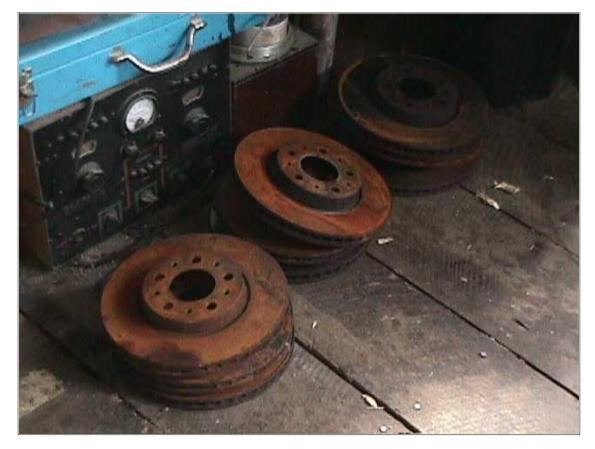
The Volvo 240 comes with 10" diameter brake rotors. I prefer a bit more diameter for a machine this large, so I found larger rotors on some of the newer Volvos - and they fit the same bolt pattern. Brake rotors on modern cars get thrown away frequently. Our local Volvo shop always has a dumpster full of them! Each machine requires 2 11" diameter brake rotors, these will be the "armature" for the alternator. Each rotor will have 12 magnets fixed to it
