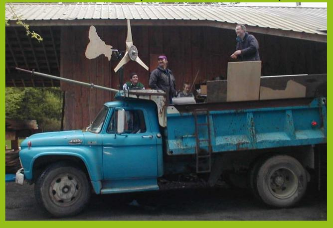
Later we did truck testing of the small machine. I recorded 30 amps output at 16 volts. But to get that output I had to hold down the furling tail and we had to hit about 45 mph. Not very scientific, but lots of fun!
