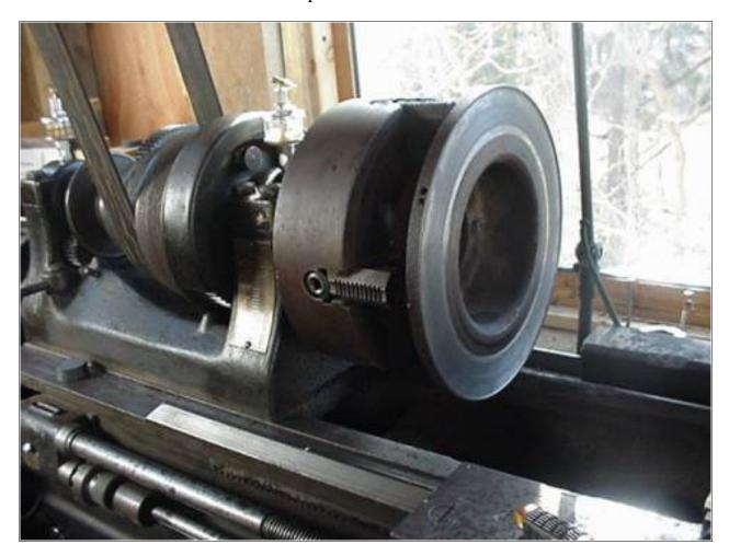
This is the only machine work involved, very easily done by any automotive machine shop, or anybody with a metal lathe. I cut a slot 1.5" wide in the back of the brake disk very near the outer edge. (I left about 1/16" steel on the outer edge) This slot serves to hold the magnets in. It might not be needed, but at high rpm there is risk of the magnets flying off. This slot should hold them in tightly.
