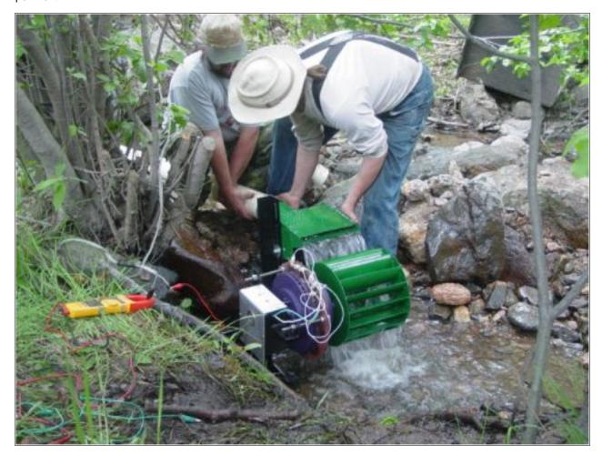
Here we've got the machine at the site, and are making adjustments. Again, just about everything is adjustable here! In the end, we got best results by feeding the water in at about 10 O'clock on the wheel, most of the water seems to exit at about 5 O'clock.
