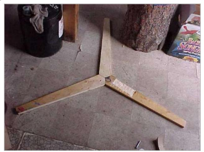
The prop is wooden, made from 1" X 4" lumber. Each blade is 3.5" wide at the base, 2.5" at the tip, and 2' long, for a total diameter of 4 feet. The pitch of the blade is 10 degrees at the hub, and 6 degrees at the tip. The hub is simply made from 2" thick wood, and glued to the shaft with epoxy. The blades are held on by one small nut at the end of the shaft, and several wooden pins. So far its held up well! Hope I never feel like taking it apart, because it would be nearly impossible...
