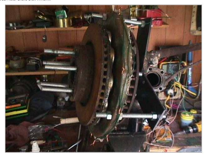
Here we basicly have the whole alternator together. At this point we could spin the alternator by hand. Were getting about twice the voltage at any given rpm now with two rotors than we were with only one before. We didn't have a tach, or even a clock with a second hand.... so no real numbers yet. But it seems to be hitting cut in voltage (12 Volts) perhaps a bit below 100 rpm.
