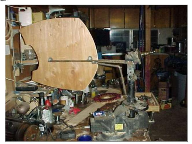
As stated above, using this assembly, with the prop canted back away from the mast - allows for a very short tail! On this the tail is supported by 2 bolts on a small frame I welded up from rhee-bar. It's very strong. The tail is cutout from 1/2" thick plywood.
