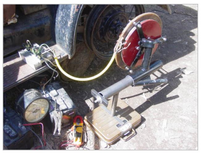
I rigged up an adaptor so I could bolt the alternator to the rear axel of my '30 Ford Pickup. By measuring output, rpm, and foot pounds I got a pretty good idea of the power curve for this alternator. It didn't seem far off the mark for a 15' prop - especially when I considered that the line from the tower would be almost 300' long. Click Here to read the whole page about testing these alternators.
