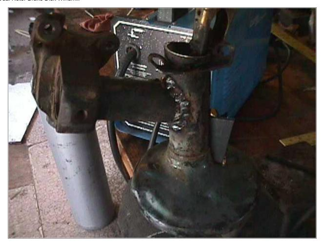
Pictured above you can see what I described a bit better. You can also see the wedge I was setting up on the back side to hold the tail pivot out at about 20 deg.
