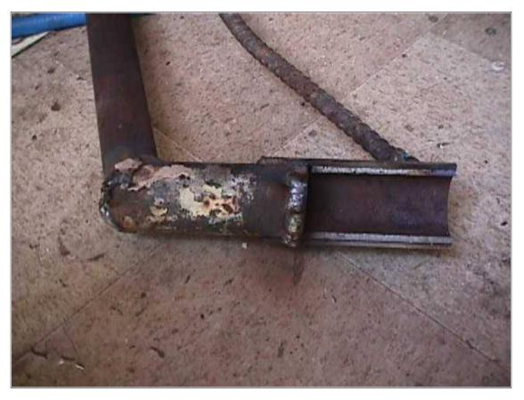
I didn't get many good pictures of this, but above is shown the notch in the tail pivot which sets the stops for the furling system. We like to weld a bead around it to strengthen it here and hopefully prevent cracking. The drawing on page one shows this to some degree. The notch must allow the tail to pivot around so that it's almost perpendicular to the wheel spindle on which the alternator rotates during furling (in high winds) and it must stop it
