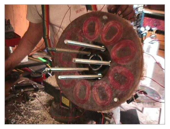
In this picture we've put the wheel hub, and bearings, and back rotor onto the rest of the wind turbine chassis. At that point we can rotate it and make sure all is flat and centered. Then we use the 3 6" long pieces of 1/2"-13
