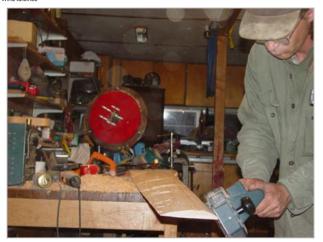
We did a lot with the power planer. I think we made over 50 pounds of chips this way! It works nicely especially on knotty wood. These boards have quite a few small knots especially towards the trailing edge. I tried to lay them out so that there would be no knots at the thickest part of the blade.
