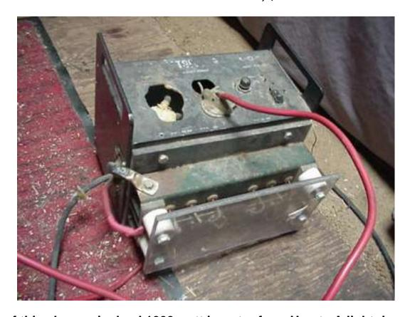
The basis of this charger is dead 1000 watt inverter from Heart. A lightning strike fried the electronics in this unit, but the transformer was intact. The owner elected to replace it with a new model, and we picked it up for \$20. The inverter case made a handy case for the charger, too, because of the handles. The whole unit weighs over 50 pounds.
