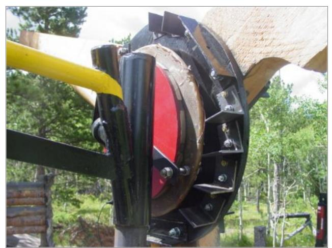
We added 1 8" wide piece of angle iron to each side of the hub on each blade, so that we could bolt through and squeeze the hub together very tightly. This made the hub much stronger. We then balanced the blade with shorter bits of angle iron and bolted them on so that they might stir some air up around the stator. After testing this alternator on the ground at 2KW output, overheating is a bit of a concern and perhaps this will help a bit.
