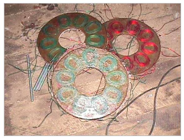
When we left off on page one we had the stator out of the mold. In this picture we have stators for 3 machines. At this point I like to chip the extra resin off the inside and outside of the stator.
