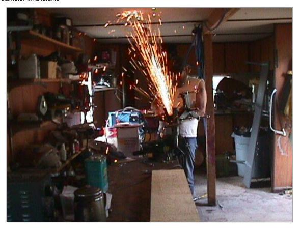
This is our last chance to grind any ugly welds down. After that we'll need to completely disassemble the machine and clean it carefully with gasoline or laquer thinner. We can then spray primer on it and paint all the metal. I prefer to leave the stator unpainted (I just think it looks neat when you can see the coils!) but we could surely paint it.
