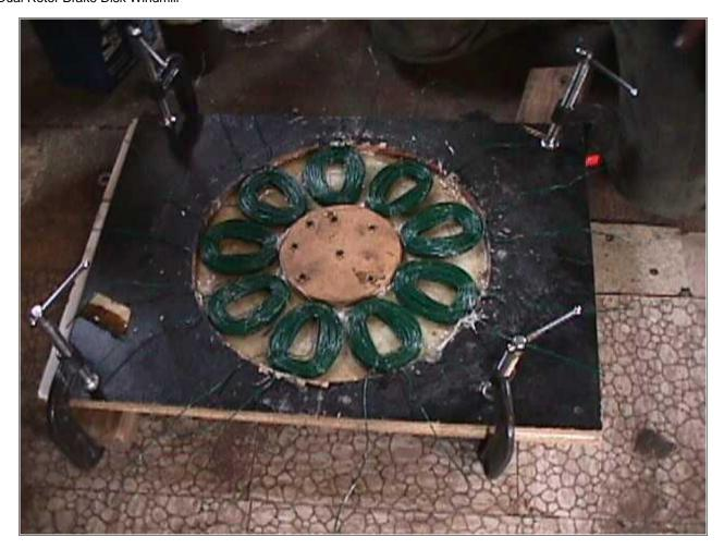
We first poured a bit of resin in the bottom of the mold (got the fabric saturated) and then placed the 9 coils in. Then we cover the coils with more fabric, and pour resin over those and put the lid on the mold.
