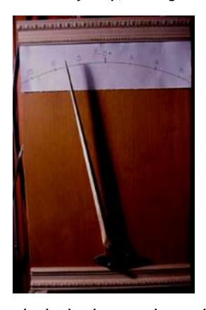
The meter consists of a wooden back, a long wooden needle(14" long), which pivots on a nail. To the bottom of the long wooden needle is a surplus computer hard drive magnet glued on with super-glue. You can get the magnet out of most computer hard drives, or...we sell them, between \$1 and \$12, depending upon the scale of meter you have in mind. (it would be great to make a BIG one)
