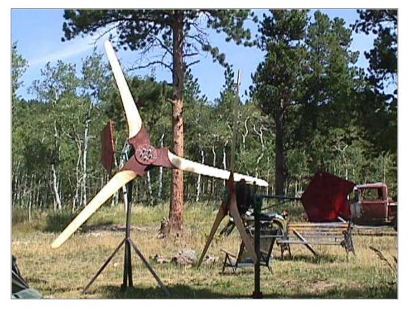
So, there it is all finished up! The only thing left to do is balance the prop, hook up the wires, and stick it up on a tower! To balance the prop we simply turn it by hand. If it seems heavy on one side, we add weights to the other side (in or near the hub). It goes quickly. For weights we used lead pipe hammered flat and held it on with wood screws. If its a slight imbalance, sometimes adding washers to the stude can get it there.
