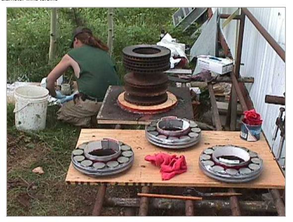
Once the resin is poured we put the lid on the mold and put lots of weight on it to keep things clamped down and flat. Best is to leave it like this overnight.... I get impatient and usually wait about 2 hours!
