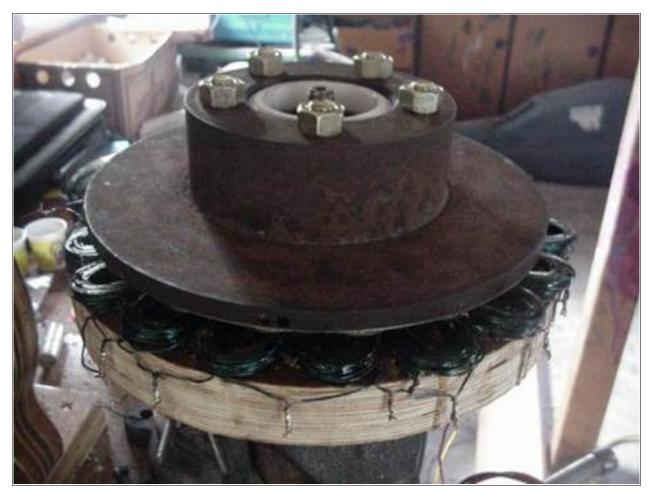
It's a radial alternator, designed around a volvo disc brake, wheel hub, bearings, and spindle. The Volvo wheel bearings make for a very tough unit, which should hopefully stand up to severe abuse! The studs which used to hold the wheel on were replaced with much longer bolts, so that the prop could bolt on the disc brake in place of the wheel. Again, please see the page about the alternator for further details about building it, and testing it - and some discussion about problems it has!
