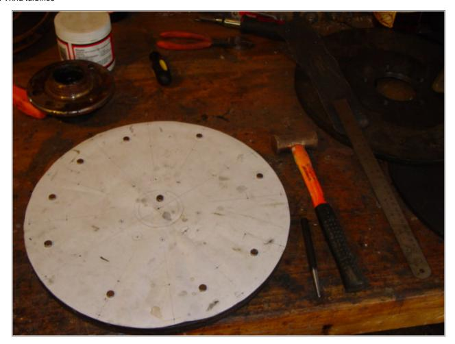
I layed out the positions for the magnets, and the holes through which the studs must fit on a paper disk 14" in diameter. I could then use a center punch to locate the holes I had to machine, and the positions for the magnets.
