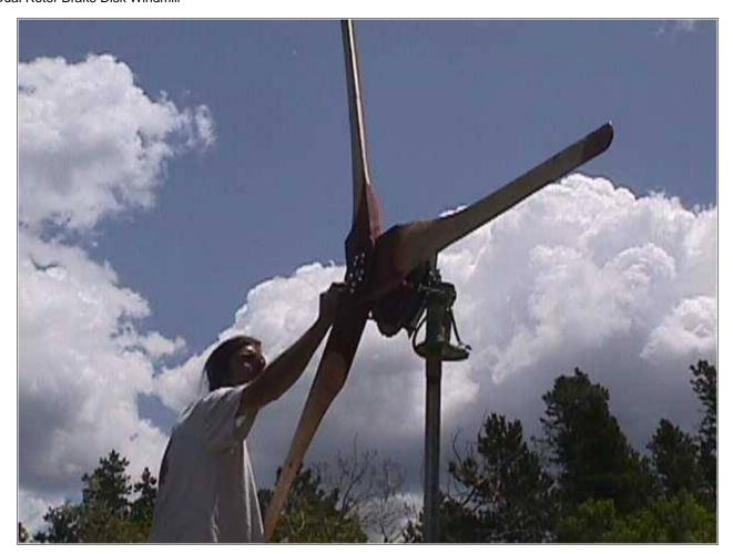
We made a short tower that fits the front of my truck. In the end, this short tower will go on top of Daves (probably wooden) tower down at the caboose. The machine weighs too much to lift it up this high, so we had to disassemble it, and reassemble it on the truck for testing.
