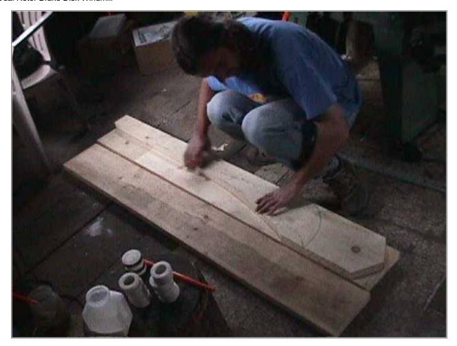
I drew up and cut out the profile for one blade, and Dave is tracing it onto blank boards in preparation for making the other two. The wood here is 6/4 (an inch and a half thick) Eastern White pine, and it's 7.5 inches wide. It's pretty lightweight, but fairly dense and strong. We have a couple knots to work around here, but not too bad.
