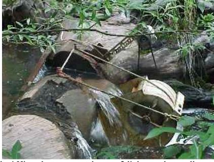
amps into a 12 volt battery, 24 hours per day! His only power needs were 2 lights, and a small car stereo, the water wheel provided more than enough. It doesn't work after the creek freezes(4-5 months of the year), and he simply lets it freeze over each year, without any apparent damage.
