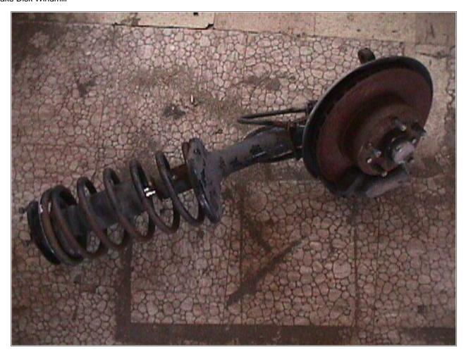
This is what I started with. It's the front strut, brake and wheel assembly from a Volvo 240. The Volvo parts are good, and since they are rear wheel drive this front assembly is simple and inexpensive from junk yards. They also built these cars for about 20 years, so the parts are easy to come by. Volvos are somewhat heavy cars, so the bearings are large and the brake disks are larger in diameter than most.
