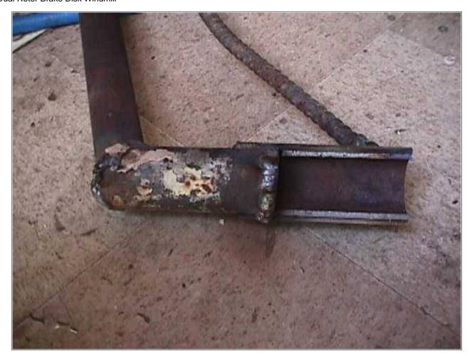
Pictured above you can see the notch in the tail hinge which determines the angle of the blade during normal operation and when it's furling in higher winds. We reinforced the pipe around the notch to make things stronger, my guess is it might crack eventually if we didn't.
