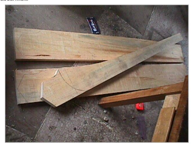
I made the blades from wood about 8 inches wide and 1.5 inches thick. Each blade started out 5 feet long, for a 10 foot prop. Here you can see I cut out the shape for one prop. Then I used it as a template and cut the others to match.
