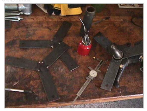
Here we see the basic frame for the windturbine with the stator brackets welded on. Now we can start really building the alternator!
