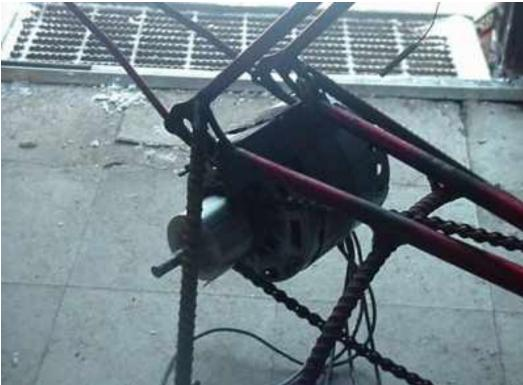
The sprocket was welded to a hub which fit the shaft of the generator. A design improvement would probably be to have a flywheel on the same shaft as the generator. The generator fit into a bracket which we welded near the back of the bike(approx where the rear wheel was). We welded "feet" together out of some re-bar left over from a concrete project. Another design improvement would be more rigid feet. The feet
