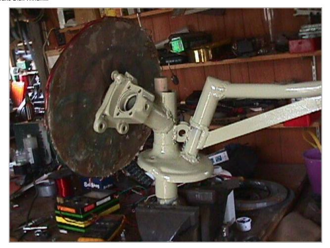
Above is pictured the main frame, with the tail mounted. I painted the metal frame with green epoxy enamel to prevent rust and keep things looking as nice as possible.
