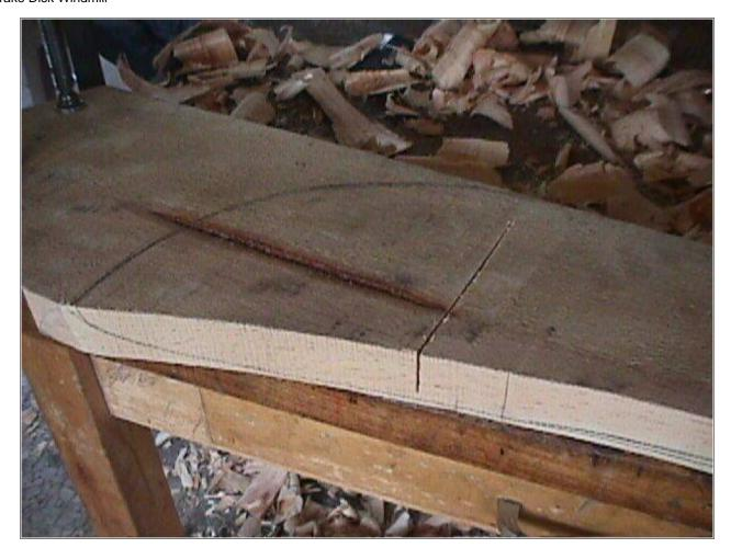
Before doing any carving, I cut one slot with a cross cut saw at the point where the angle of the blade is steepest. This is insurance that I won't ruin the hub area of the blade with the drawknife should I make a mistake or have the wood split.
