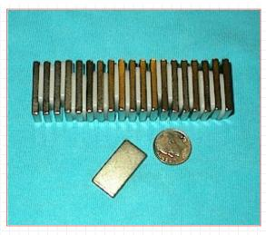
More Neodymium magnets for those on a budget. They make nice alternators as shown in the section "Alt from scratch"
