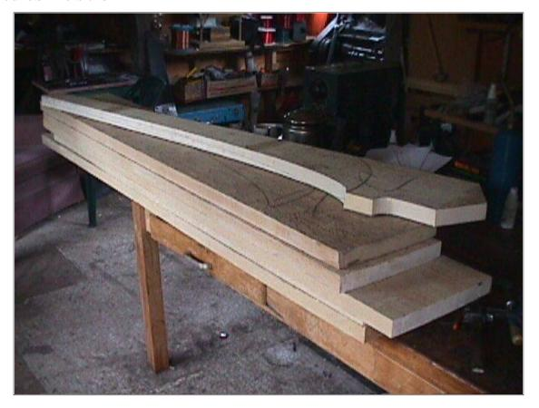
We start with boards which are 5' long, about 7.5" wide and nearly 2" thick. I layout the shape of one blade, and cut that out. Then we have a template to trace around.
