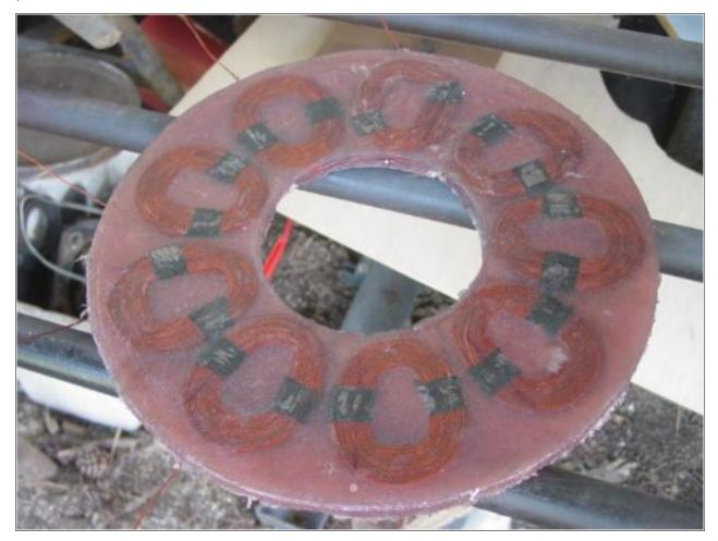
Pictured above is how the stator looked after casting. It's 14" diameter, and 1/2" thick... it came out nicely.
