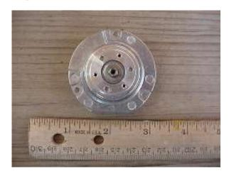
Surplus brushless DC motor used for the ball bearing inside and easy mounting
