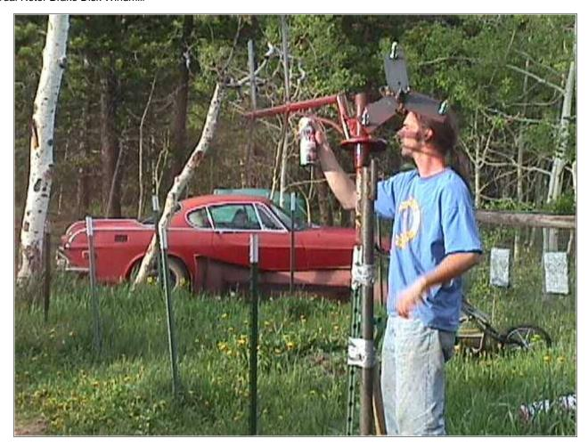
Here Dave is putting primer on the machine. First we ground off some of the uglier welds and then cleaned it carefully with gasoline to remove any oil.
