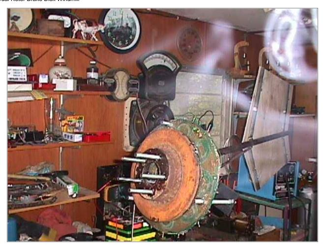
Here the alternator is pretty much done, and the tail is finished! The tail occupies between 5 and 6 feet of area. (If you look real close at the ammeter on the wall, you can see that my <u>last wind turbine</u> is putting out about 40 amps. It was a breezy day!)
