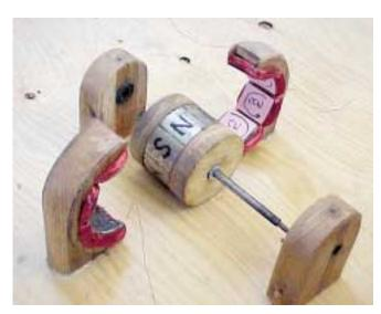
An exploded view shows the armature, stator, and pillow blocks ready to assemble into an alternator.
