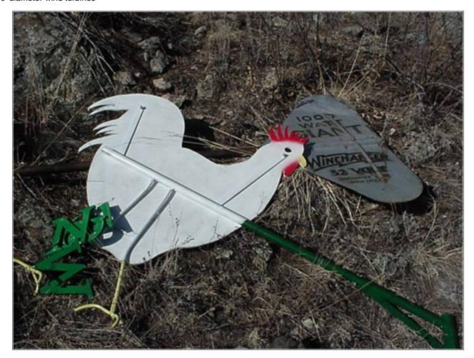
Here we have the tail up on the site where we raised the machine. Beneath it is the tail for his antique Windcharger Giant, which was origionally a 32 volt machine with an 11' prop. His was always missing some parts and he was running a belt off the blades to a PM DC motor which worked out OK, but it had some problems and we replaced it.
