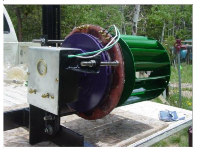
Here it is all painted up! We'd intended to put a shroud over the alternator that would rotate with it, to keep water out of the bearing and off the electric components. We never found the right piece and ran out of patience with that, but we will add that later if it works well enough to warrent the effort.
