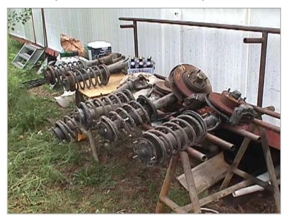
Pictured above are the Volvo 240 strut assemblies we start with. Volvo made the 240 for almost 20 years! They should be easy to find. We have to remove any extra parts that come with the strut assembly.
