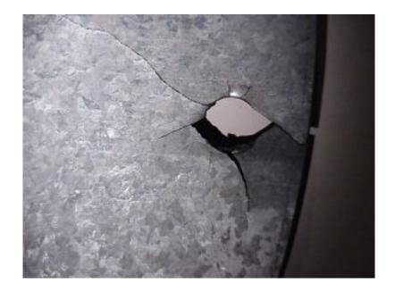
Stress fractures from vibration in a sheet metal tail. We don't use sheet metal any more because of this...can you see why we think sheet metal blades are dangerous?!?!
