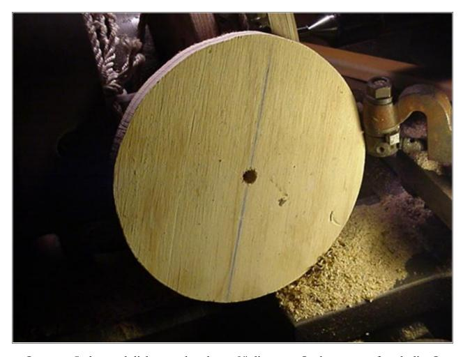
I cut out 5 plywood disks on a bandsaw, 9" diameter. In the center of each disc I drilled a 1/2" hole. These disks are laminated on the shaft to build up the armature. In order to hold the armature securely to the shaft, I drilled a hole about 4" from one end
