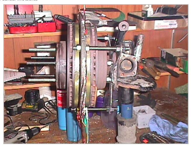
Just another alternator made using the volvo 240 strut tower, and brake disks. Again, we've put 12 2" diameter X 1/2" thick magnets on each rotor. Georges coils are wound with 35 windings of #12 wire, and the stator is wired in Star. This is somewhat of an improvement over the earlier machines which we had wired in Delta.
