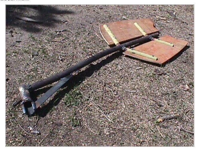
The tail is shown above. Actually - when I got 'round to testing this the tail came up too small and too light weight. I wound up making it slightly larger in the end. The end which attaches to the wind turbine is a short segment of pipe slightly larger than the 1 inch diameter pivot, which is welded to the main frame of the windmill.
