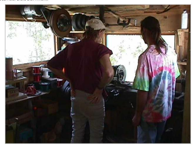
I like to cut the brake rotors down so that there is a slight lip (about 1/16 inch) to hold the magnets in. This helps a bunch too in spacing the magnets out evenly later. Pictured above Dave is doing this on the lathe.
