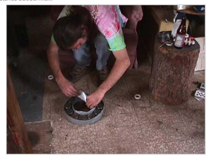
Here Dave is putting duct tape around the inner and outer diameters of the magnet rotor. This simply serves as a "quck and dirty" sort of mold, so that we can pour the resin around the magnets and it hopefully wont run out the sides!
