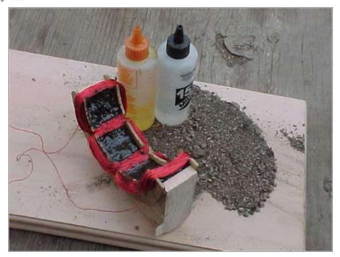
The dirt was mixed with epoxy, so that I had a thick paste. I simply spooned it inside the hollow space in the stator. This makes for a reasonable core, and although it does not work nearly as well as steel laminates, it's much easier. Making steel laminates is a nearly impossible task without significant time and tooling. The magnetite paste does a good job of attracting the magnetic field, and is non-conductive so eddy currents are not a problem.
