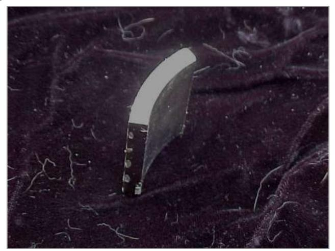
Pictured above is one of the magnets I used. These are surplus magnets from computer hard drives, one of my favorites for alternator experiments. They are about 1.75" long, 1.4" wide, and a quarter of an inch thick. 8 of them will fit together to make a ring. We no longer have these magnets in stock. They were surplus, they are sold out, and we can't get any more. But this design could easily be adapted to use different size or shape NdFeB magnets.
