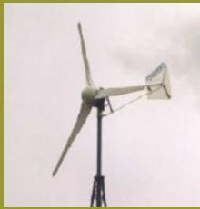
The wooden blades of the original were replaced by fibreglass, and the tail was simplified.
