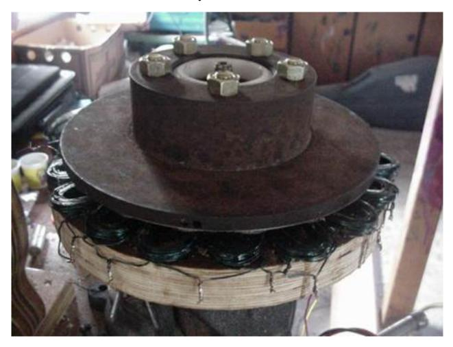
Homemade Volvo Brake Disc PM alternator, 800 watts, \$150!
