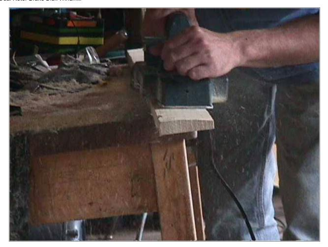
Here we are finishing up the front of the blades with a power planer. We did most of the work with the draw knife, but the power planer does nicely to finish things up quickly.
