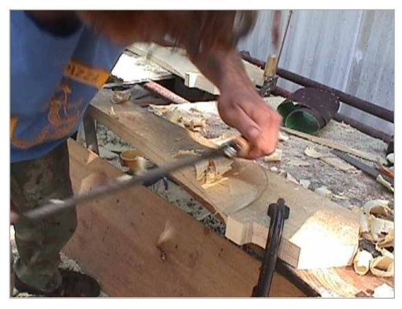
In the picture above I'm carving down to the line. This goes really quickly with a sharp draw knife.
