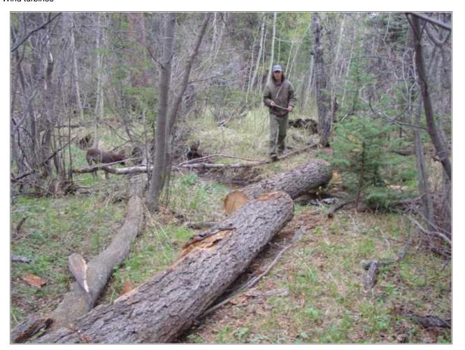
The first step was to cut it into 10' long sections. Although we didn't see many knots at this point, I figured there might be some. I could also see some rot just under the bark, so I figured we'd do well to have them a little longer so we could pick the best part of the boards.
