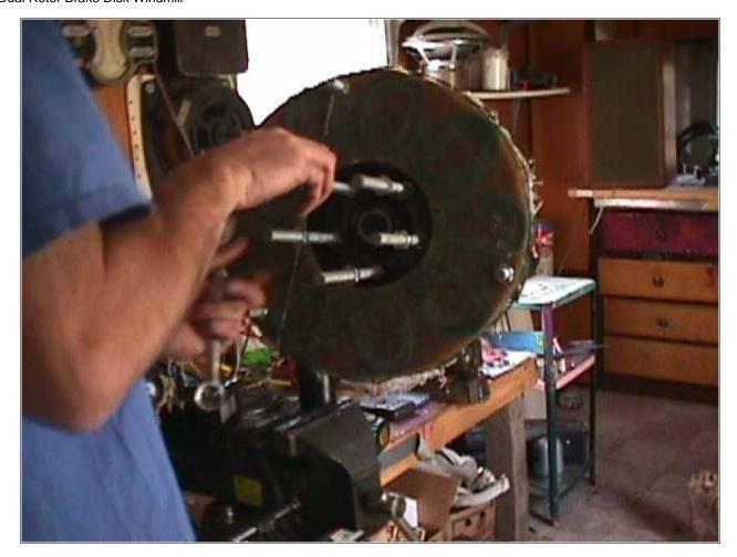
Here Dave is putting the stator on over the first magnet rotor. It's interesting to note here... with one magnet rotor on the machine, and the 3 long pieces of steel allthread which hold the stator on, that the magnets are somewhat attracted to the allthread and at this point the machine cogs a bit. When we attended <a href="Hugh Piggot's seminar in Guemes">Hugh Piggot's seminar in Guemes</a>
