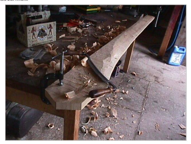
After attending Hugh's seminar this spring... the drawknife has moved to the top of my list as the favorite tool to use. Very fast, and very accurate. No need for a chisel and the only power tools were used for finishing. I roughed out the whole prop with this quickly and then finished it up with a power planer and a belt sander.
