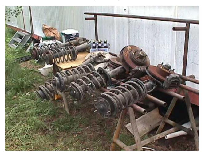
Again, I started with the strut tower from an old Volvo 240 sedan. Here, the main part we're using is the wheel spindle, the hub and bearings, and a bit of the tubing.
