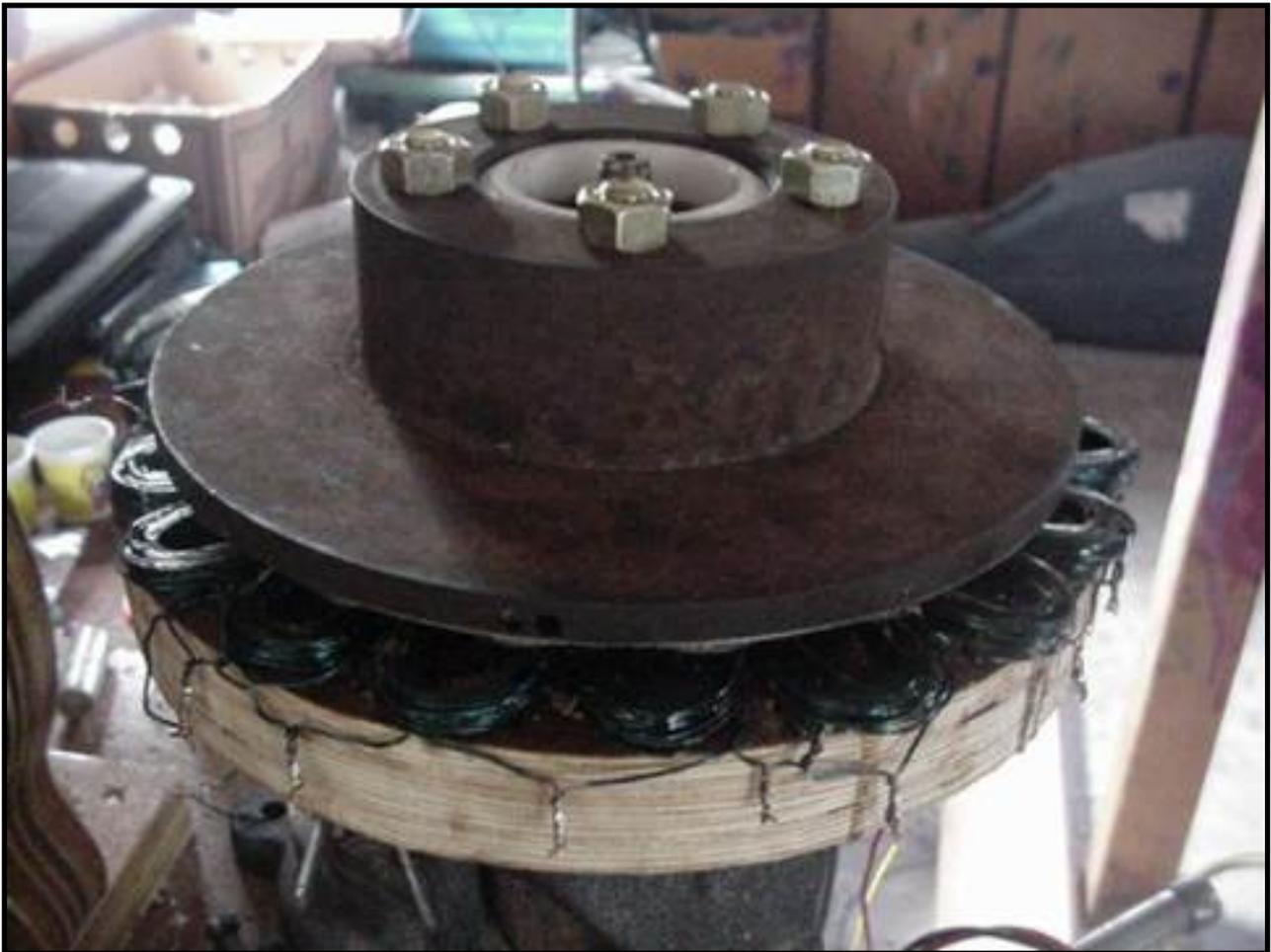
It's a radial alternator, designed around a volvo disc brake, wheel hub, bearings, and spindle. The Volvo wheel bearings make for a very tough unit, which should hopefully stand up to severe abuse! The studs which used to hold the wheel on were replaced with much longer bolts, so that the prop could bolt on the disc brake in place of the wheel. Again, please see the page about the alternator for
