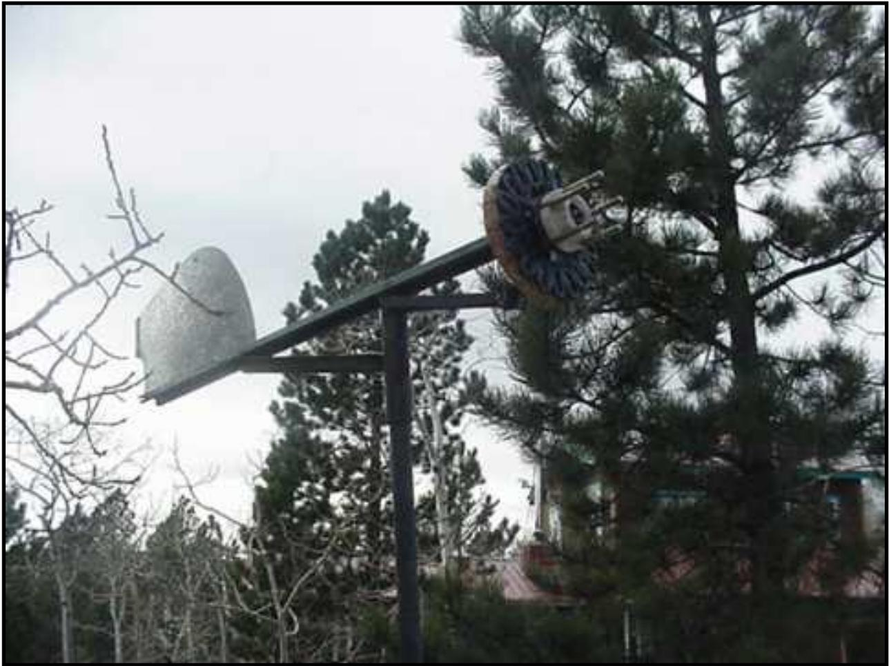
The tail I cut from thin sheet metal, which is bent, and folded over on the back side. Since I have no tin snips, we cut the tail out with an angle grinder. The tail is bolted to the signpost, and 1 heavt steel bracket is bolted to the top of the tail for reinforcement. As it turns out - this is inadequate. I've seen this machine running now for a couple weeks, the tail is NOT longed for the world. It should have been much stronger. We'll take it down soon and fix it.
