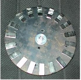
The magnet rotor will be mounted to the prop hub and the stator will be attatched to the bearing head. To complete the rotor the magnets are glued in place and resin will be poured onto the plate to lock them in forever then it will have to be balanced.
