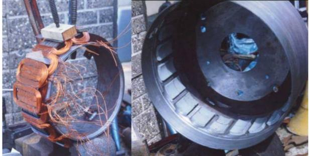
The 20 magnets Les used are also neodymium ones, with a rather unsuitable curve on them, but they are nicely fitted to the rotor by painstaking machining.
