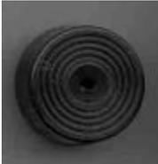
A piezo buzzer uses the piezo electric effect to convert electricity into motion of a thin slice of crystal material. With enough voltage, the piezo buzzer will make an audible sound. The experiments in this plan use a piezo buzzer because it makes it easy to “hear” that a current is alternating or not, and even how high the voltage is (by how high the frequency sounds).
