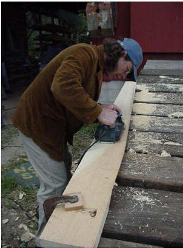
DanB running the planer on a blade for the new 12-foot machine design. The blades are Yellow Cedar, which cuts pretty well with a drawknife...but the turbine blades are BIG and the planer did speed up the process somewhat.
