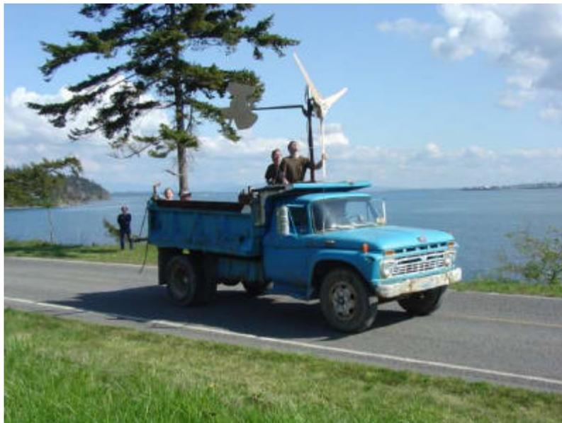
This is not really a very good way to test wind turbines. But it is FUN, and you can start getting an idea of how the alternator performs and when the furling system starts to kick in. Don't rely on windspeed data when truck testing, though -- whether it's from the truck speedometer, an anemometer, or a GPS unit, windspeed readings will be skewed by the airflow around the vehicle.
