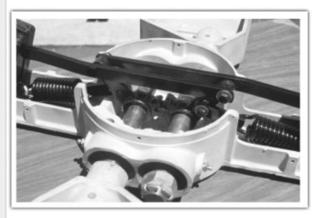
(Above) At rated speed, the governor's weights arc outward, pulling the gears and prop shafts into rotation, preventing rotor overspeed.
