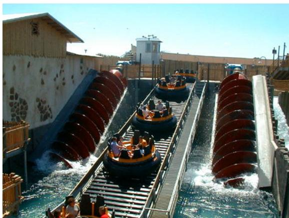
Fig. 5 Archimedian Screws installed in a theme park (29)
