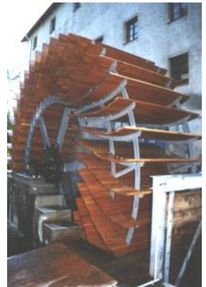
Fig. 12 above Sketch of installed Zuppinger wheel (27)
