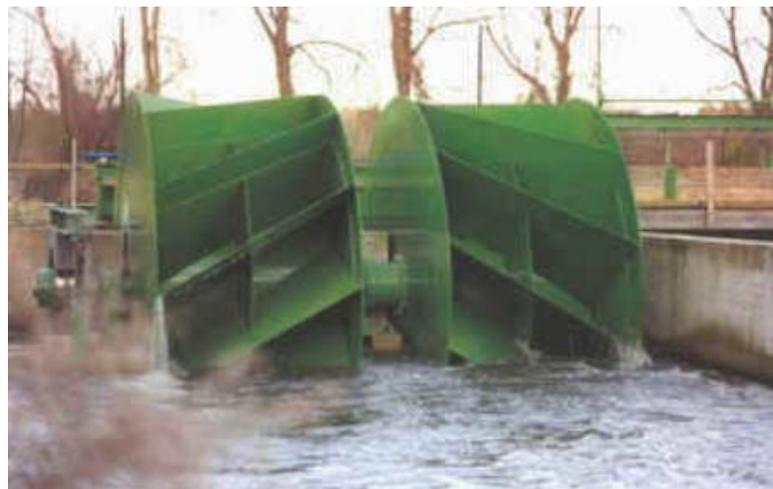
Fig. 18 (above) Photo of Staudruckmaschine installed (45)
