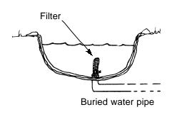
A simple holding tank: a bowl-shaped hole in the ground, lined with six or eight mil plastic sheeting. You can line the hole with cardboard or old carpeting to protect the plastic.
