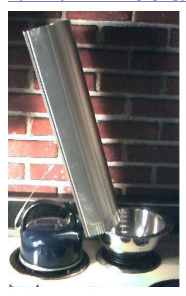
It is easy to produce way too much steam and overwhelm the cooling area, which needs to be as large as possible. If one produces too much steam it keeps the condensation area hot all the time and thus no condensation takes place. One will not be able to regulate the source of heat in a primitive environment thus this method could be a problem.
