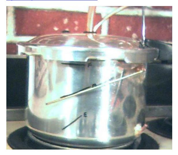
It was made out of a large inline disposable gas filter with the ends cut off and soldered up to make it air tight. See <a href="http://home1.gte.net/mikelob/Float-Hing-1.JPG">http://home1.gte.net/mikelob/Float-Hing-1.JPG</a>.
