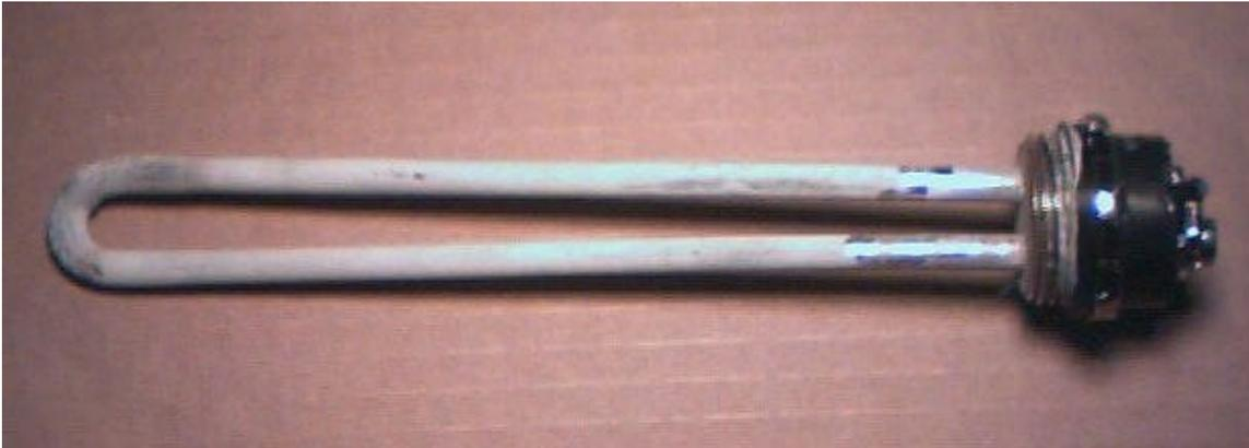
Warning: Running the eclectic heat element without water only lasts for a mater of seconds before the heater element burns out. It makes a popping nosed which is not all that laud. Changing out the heater element is the only thing that can be done to fix this. Cost is about \$8 at Home Depot. You may want to stock up on as many spares as you can afford.
