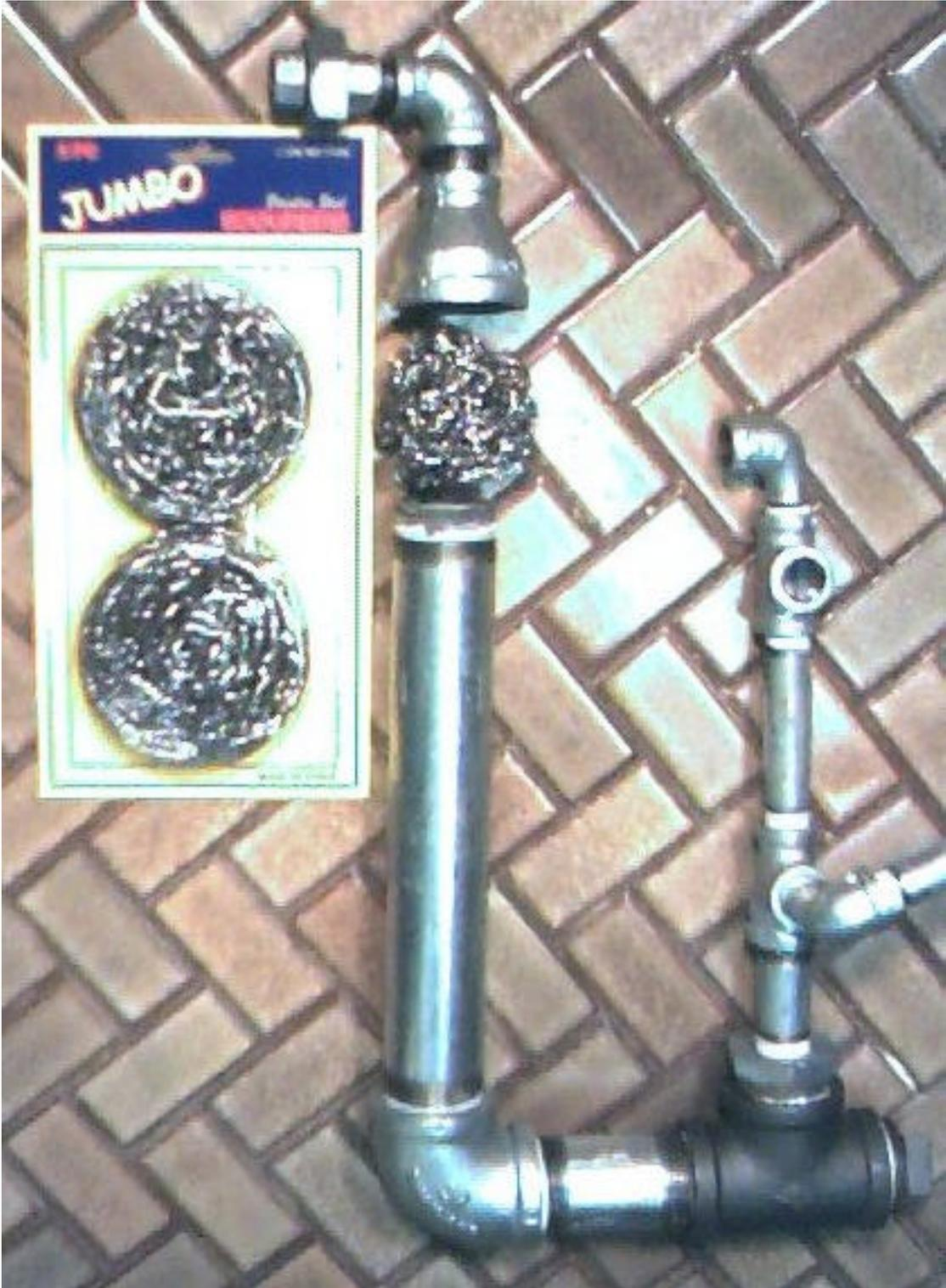
During the construction process cut in half a heavy duty stainless steel scouring pad (the coarser the better) and stuff this into the end of the steam 1.5" pipe at the reducing
