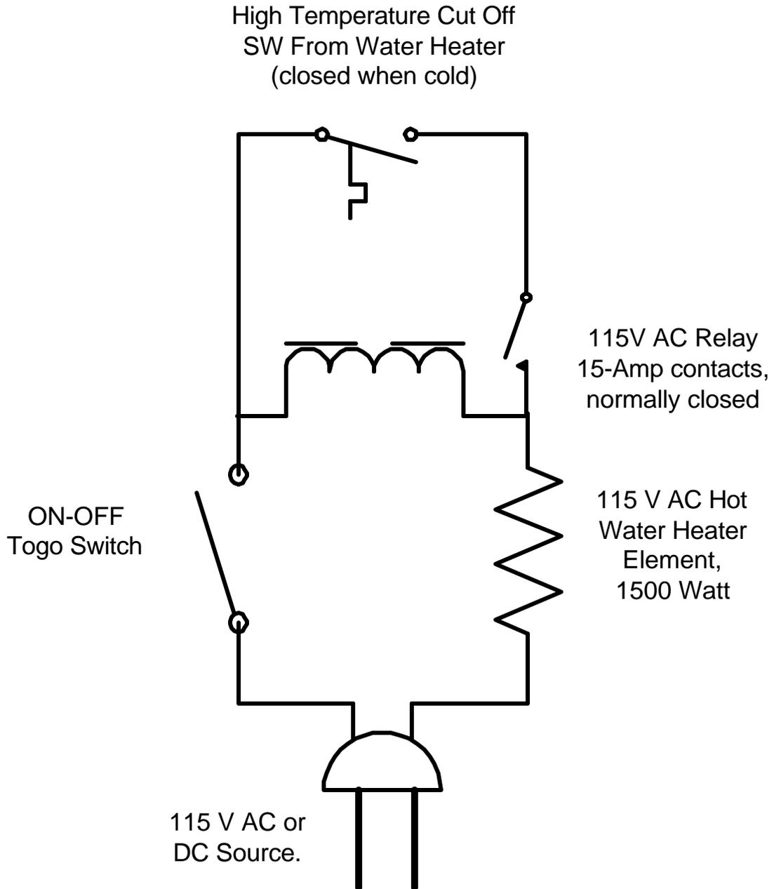
If the cooling flow stops then the temperature switch will turn off the current flow to the heater element. If the water flow stops totally then about 40 sec latter the 150 degree F
