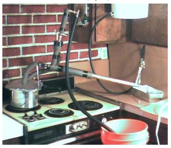
6) When the parts are available after a PS this sort of approach will work. It tends to be a batch operation that needs close attention and potential continuous maintenance. <a href="http://home1.gte.net/mikelob/Coil\_Exchanger.JPG">http://home1.gte.net/mikelob/Coil\_Exchanger.JPG</a>
