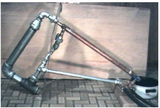
5) Pressure cooker and straight pipe heat exchanger type of water distiller has the advantage of being able to mix more air and potentially releasing more hydrocarbons from the replenish water then any of the above four approaches. A bit more difficult to keep the replenish flow rate adjusted during operation than the other. <a href="http://home1.gte.net/mikelob/Exch-full-Inso.JPG">http://home1.gte.net/mikelob/Exch-full-Inso.JPG</a>
