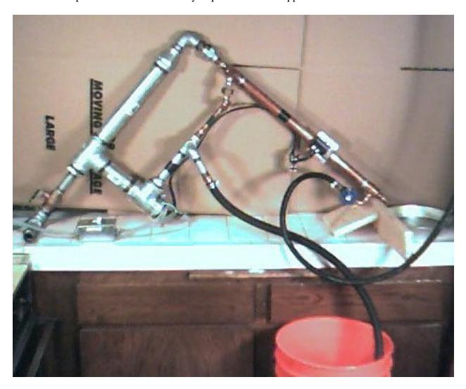
2) & 3) The Light and Heavy Duty Pots & Pie-Pan water distiller has the advantage of portability and ease of construction. They both produce a relatively high amount of output and have flexibility as to the source of heat. Safely empting the hot cooling pot at the end of each batch (about every 40 min) is the only danger to the using this approach. See <a href="http://home1.gte.net/mikelob/WDL-2.jpg">http://home1.gte.net/mikelob/WDL-2.jpg</a>
