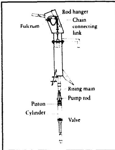
are willing to apply for progressively less water as depth increases. The submerged cylinder eliminates the need for priming, but means that repairs or maintenance involve removal of components from down the well.
