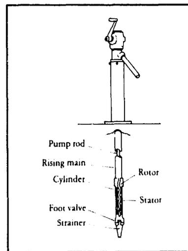
vertical plane into a horizontal plane rotation of the pumprod (a direct-drive version with the handle rotating in a horizontal plane is also available). One advantage of rotary pumps is that they are simply converted to motorized or animal power. On the other hand, the rods and rotor assembly need special lifting equipment when installed in or removed from deep wells.
