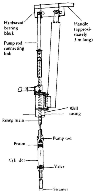
a concrete foundation block that also encompasses the borehole casing. The handle is made from 2-inch galvanized steel pipe and is typically 10 to 12 feet (3.0 to 3.7m) long with a single bend. In this way the upward travel of the piston is limited by the handle contacting the ground.
