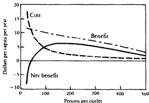
optimization is needed for that option. Once the best configuration for each type of system has been determined, handpump, standpipe and yardtap systems can be compared on the basis on net benefits.
