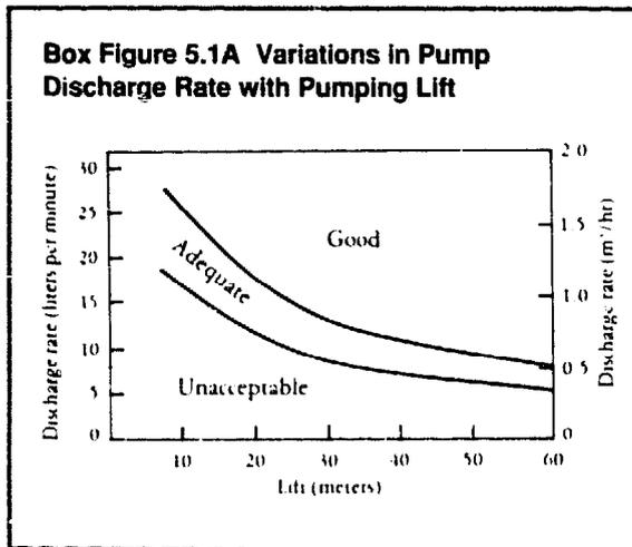
lift of 7 meters and increasing to 75 watts at a lift of 45 meters or more. Adults will usually apply over 100 watts (and sometimes over 150 watts) at high lifts in order to increase the discharge rate. A representative range of mechanical efficiencies has been used — from 45% at 7 meters to 70% at 45 meters. "Good"
