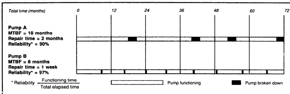
The "**reliability**" of mechanical equipment is commonly measured in terms of the "mean time before failure" (MTBF). Thus, Pump A which has a MTBF of 18 months would be judged to be more "reliable" than Pump B for which the MTBF is 8 months.
