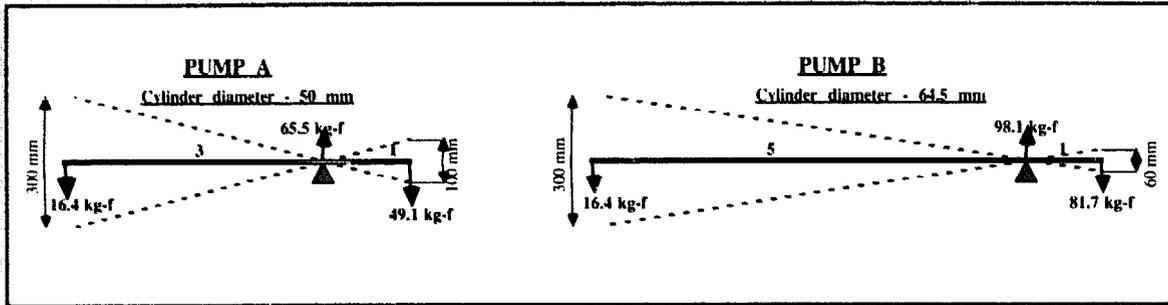
Field trial observations have shown that users of lever-action handpumps tend to move the handle end by the same amount irrespective of the total stroke length available. This constant travel distance (usually in the range of 300 to 400mm) is maintained as long as the operating force is within acceptable limits. This finding has considerable significance for handpump designers.
