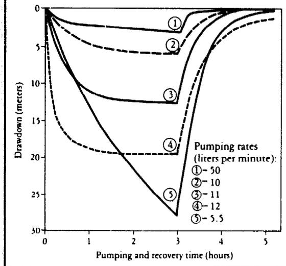
such as permeability are often more important than the pumping rate in determining drawdown, as evidenced by Curve 1, where the well with the highest pumping rate has the least drawdown.
