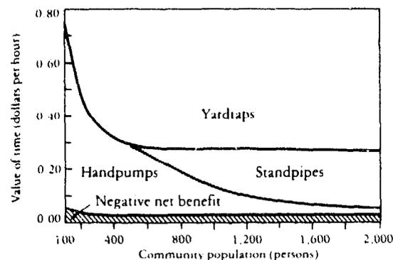
Note: These graphs apply to diesel pumps for standpipes and yardtaps. Unless otherwise specified, pumping lift = 20 meters, well cost = \$2,000 per well, population = 400 persons, and housing density = 25 households per hectare.
