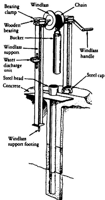
particularly well suited to VLOM (Village Level Operation and Maintenance). A major disadvantage of the Bucket Pump is the low rate at which water can be extracted from the well, making it more of a family or multi-family pump and not suitable for use by larger numbers of people. Another disadvantage is that some contamination may take place.
