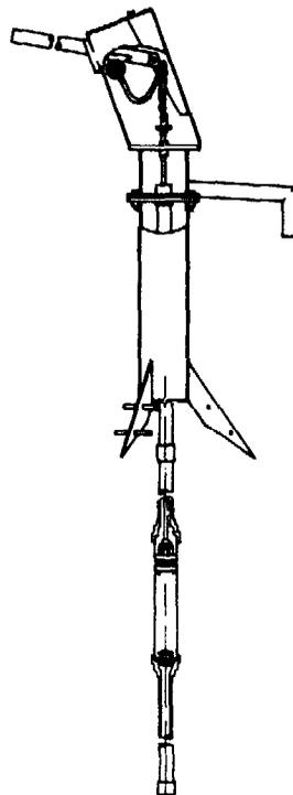
India Mark II. The Sholapur pump was strengthened and the solid bar handle for counterweighting was added. Various other design changes made it possible to mass produce the pump in simply equipped workshops, to make it easier to maintain, and to prevent tampering. At present, there are 36 manufacturers certified to make the India Mark II.
