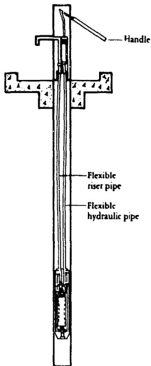
bicycle drive. The pumphead contains a hydraulic unit connected by flexible pipes to another diaphragm pumping unit below ground claimed to be capable of producing over 8 liters per minute from 80 metres. This pump is expected to be tested at CATR laboratories during 1987.
