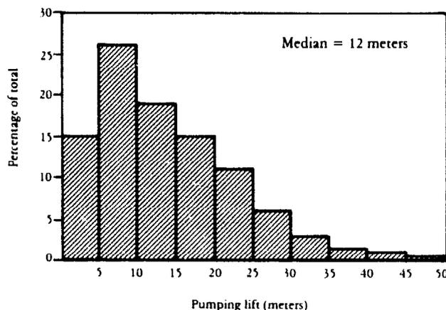
*In the Project field trials, efforts were made to site wells where groundwater was as deep as possible — the aim being to develop handpumps suitable for deepwell applications. However, as the diagram shows, 75% of the wells involved pumping lifts of less than 20 meters, and 85% were less than 25 meters. It seems likely that these figures are a good reflection of the global situation in terms of groundwater depth.*
