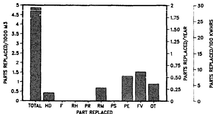
HD-Handle RH-Rod hanger RM-Rising main PE-Pumping element
