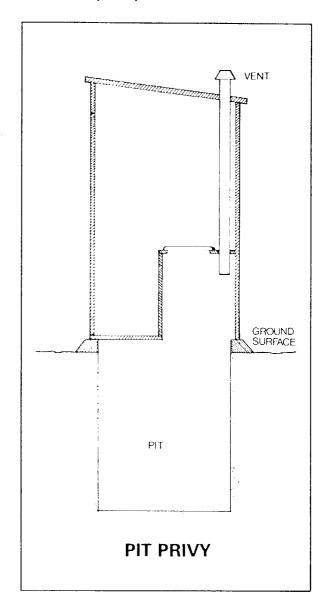
on the top of the vent pipe will discourage flies, and a little raised roof (not a lid) will keep out the rain. The Ministry of the Environment supplies a working drawing on request.
