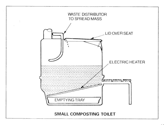
with the out-of-doors. When all goes well, this vent is not merely a passive conduit, but a chimney. The composting material in the tank is warm, as are the water vapor and carbon dioxide rising from it. As warm air rises, the column of warm gases in the vent pipe flows out the top of the pipe.
