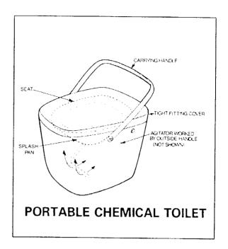
carried with some care to avoid splashing or spilling. Its capacity is, of course, limited by the need for portability, and the usual requirement for safe disposal of the contents remains. These units may be drained into a standard toilet and flushed to municipal sewers, but not to a private septic tank.
