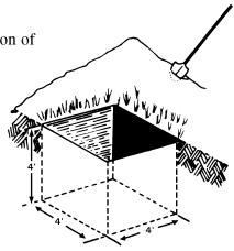
Soakage pit/trench—Used to prevent accumulation of liquid waste (water
