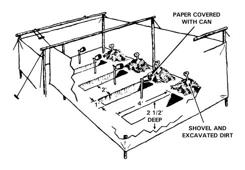
• **Deep pit latrine**—Used for longer periods of time and in built-up areas. Collapsible two-seat boxes are available in the supply system.
