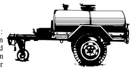
from the tank. Foul odors, bacteria growth, and rust will accumulate during storage if the water is not completely drained.
