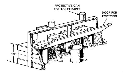
• **Burn-out latrine**—Use where water table is too close to the surface of the ground for digging a pit latrine, or stay is for an extended period.
