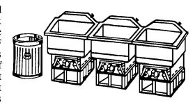
Scrub mess kit in the warm, soapy water by using a long-handled brush. Rinse the mess kit in the second sink of clear, 170° F water. Disinfect the mess kit by immersing it in the third sink of 180° F water for 10 seconds. Air-dry mess kits.
