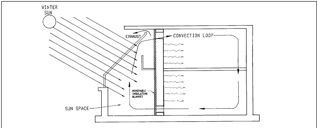
Figure 2. Isolated gain system using a sun space
