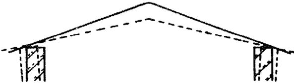
1. Figure 1 shows that a roof construction of only rafters tends to spread the walls. This is because the roof doesn't have a triangular shape, so it is not a perfect structure. This construction could cause damage to the walls, the roof, and the whole building.
