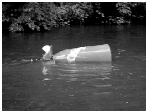
Figure 9. Operating Sling Pump
