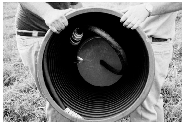
Figure 11. Inside of Sling Pump
