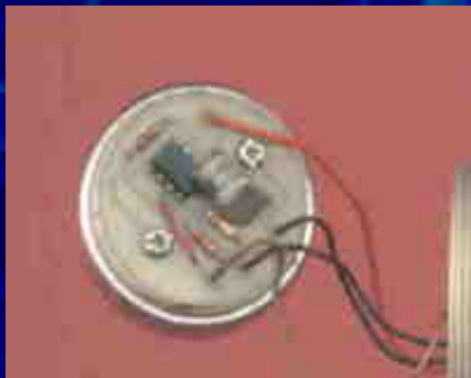
A view of the circuit board attached to the receiver. ( Back )
