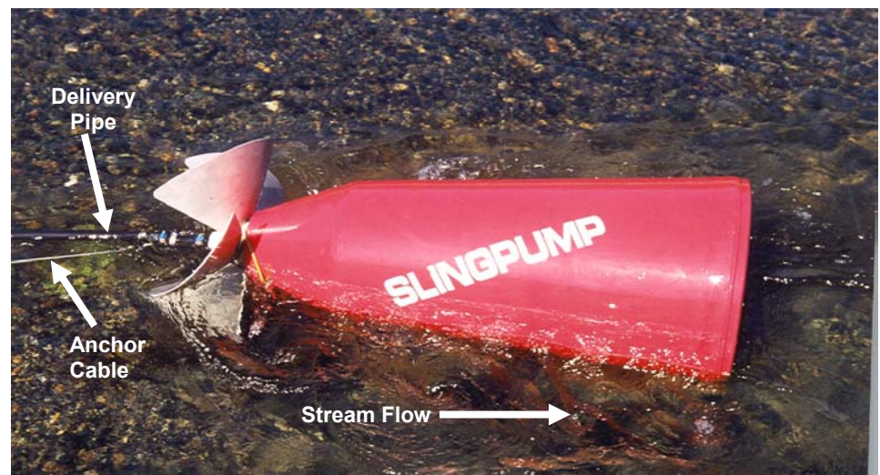
Figure 2 Sling Pump Operating in a Stream
