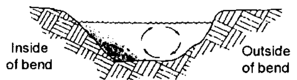
Section through river on a bend
