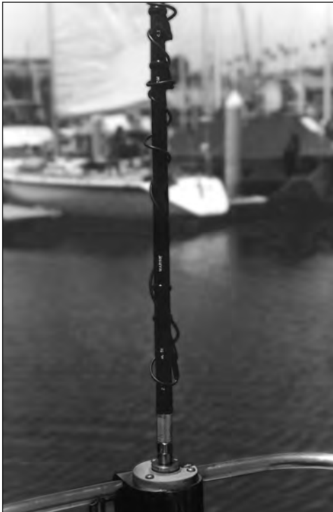
Whip antenna mounted over a stainless steel rail
