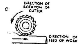
Distance between the side milling cutters adjusted to machine dimension "A" within its tolerance
