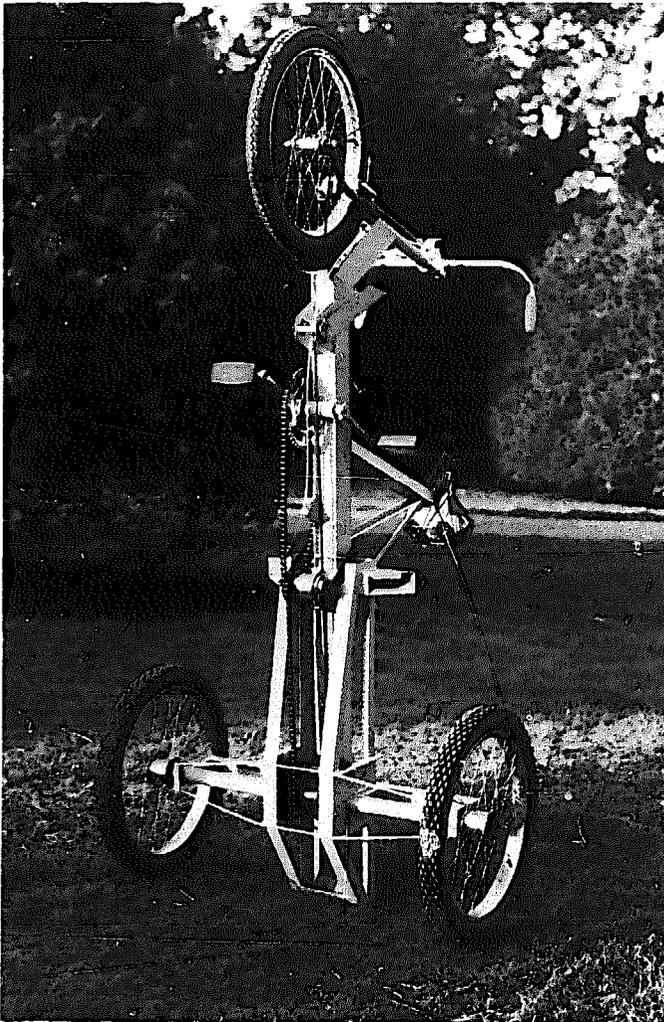
**Figure 2-5** Up-ended view of Oxtrike chassis showing ability to park in a small space, easy inspection of transmission and brakes, and ability to tip out the load. Note Sturmey-Archer three-speed hub gear with double adjustment for primary and secondary chains.
