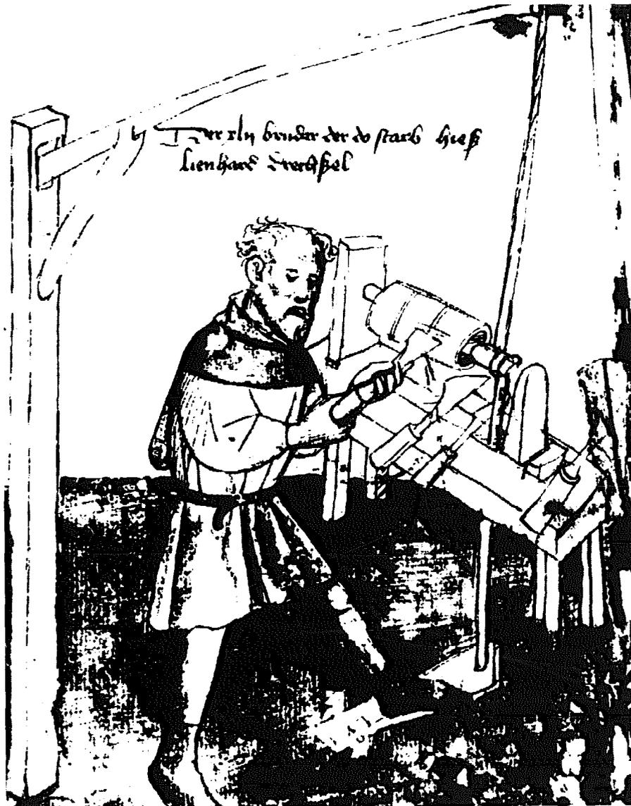
Figure 1-18 Foot-powered lathe (Courtesy of Friedrich Klemm)
