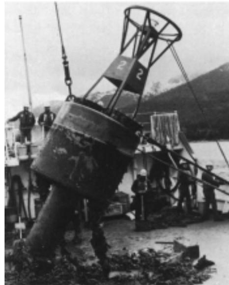
Figure 509. Buoy showing counterweight.
