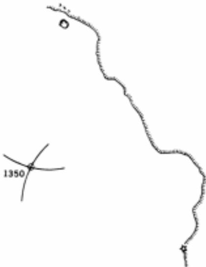
Figure 811b. A fix by two radar ranges.
