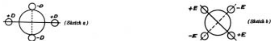
Figure 607. Summary of compass errors and adjustments.
