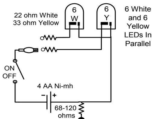
Hook Clip to -12 V DC turn on the switch and + Terminal to charge the 4 AA cells
