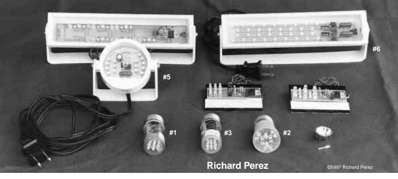
ere is a lighting test—which lighting technology can produce the most light for the least power? The hands down winner is the light emitting diode (LED) which makes three times more light per watt than a compact fluorescent and 30 times more than a standard incandescent.
