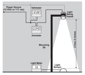
standards have been met. The Greenlee reads out in foot-candles. The distance from the lamp to the light sensor on the Greenlee was 2.5 feet (0.77 meters). I made the electrical measurements (voltage and amperage) using two Fluke 87 digital multimeters.
