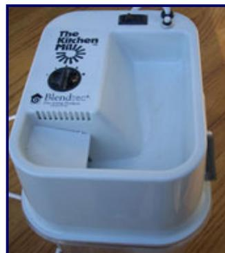
On the downside, the blades are fragile, and small rocks or pieces of metal can damage the wheels. If you have an impact grain mill, be sure to use only grain that has been well-cleaned (for example, commercially purchased grain).
