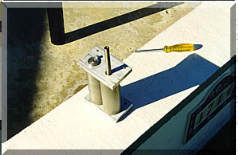
The draft plate, a very busy part of the mill, is constructed from a piece of 3/4"X6"X18" oak board and has a 1 1/2"X5 3/4" rectangle opening in it used to draft the malt into the rollers. It also is used to attach the mill to a workbench or to set atop a plastic bucket. Further this board provides lateral spacing of the frame.
