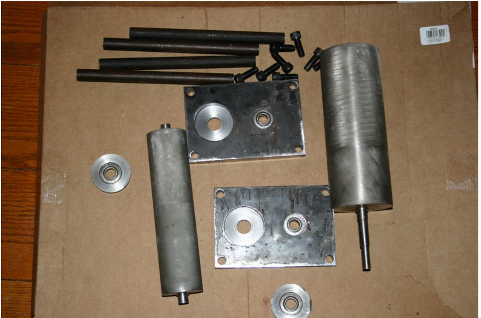
The mill easily goes together in a matter of seconds. I ended up priming the carbon steel and washing the rollers after my first experiment. I'll probably use it a few times before I actually paint it. I'm thinking a nice chrome would look nice with a clear finish over it. I'll probably wait and get the cheapest paint I can find, once again reducing cost. The stainless rollers will never rust, but the rest of the body might not like moisture.
