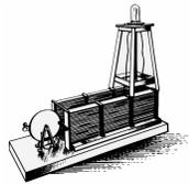
**1832 ~ FARADAY** demonstrates a large version of his first continuous uni-directional electric current generator apparatus, by using the large horseshoe magnet at the **Royal Institution**. (**Note:** This demonstration concerned a homopolar apparatus that was "**not**" acyclic in its nature of operation.)
