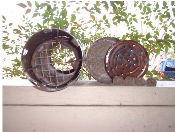
Looking from the bottom (top is unchanged), both bottoms have been cut out and  $\frac{1}{4}$  inch hardware cloth has been shaped and inserted in the base of the burner. The church key tabs made from the can opener, on the cowling, have been bent down  $180^\circ$ . These rest on the rim of the ash holder (right), which provides a stable base for the stove.
