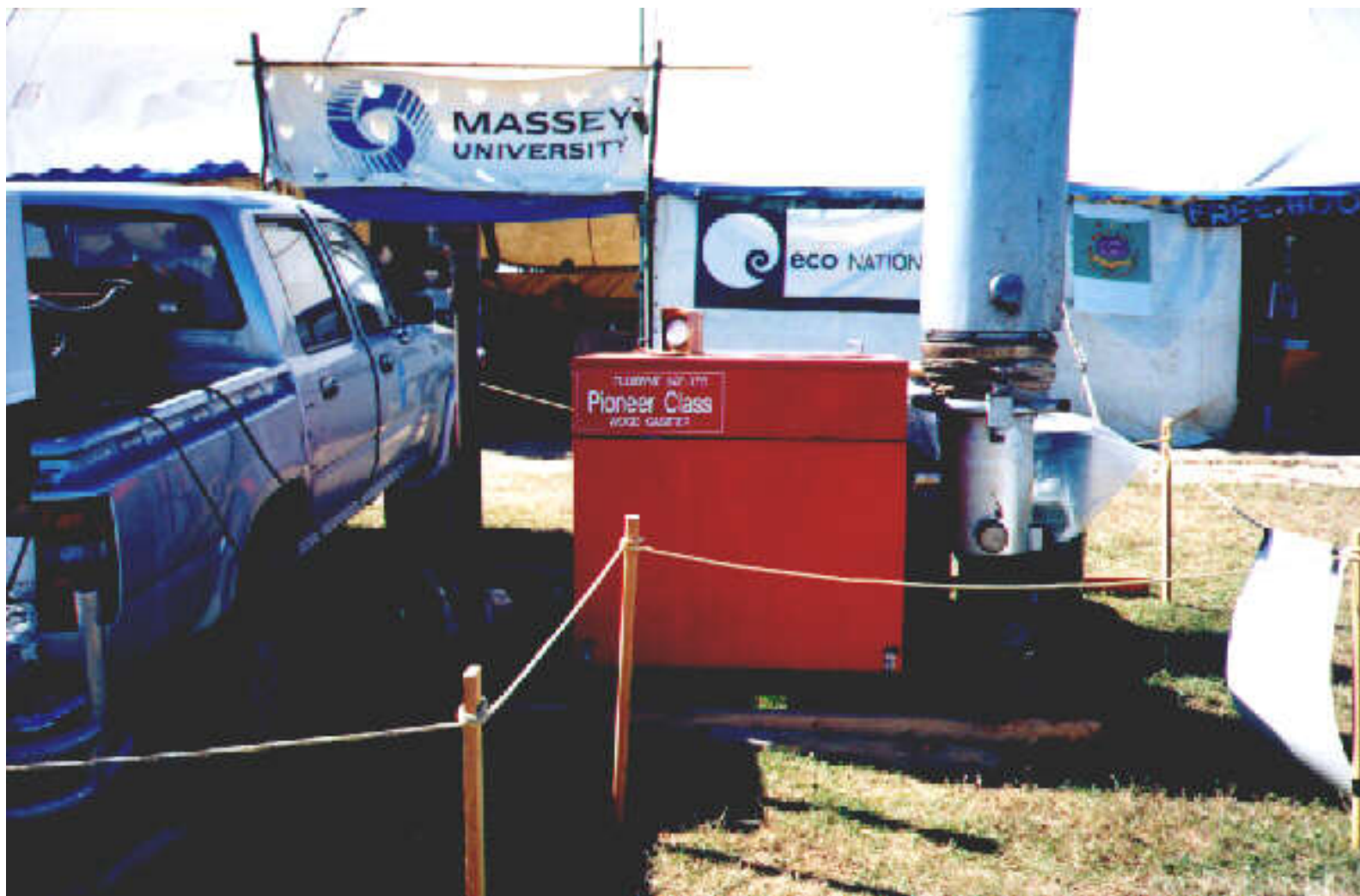
The Pioneer Class gasifier.
