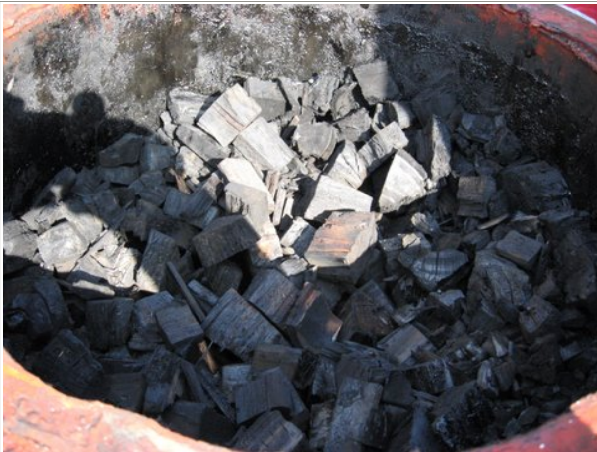
IMG_0229.jpg 15. At 50mm above the air nozzles, the raw wood has almost completely turned to char.
