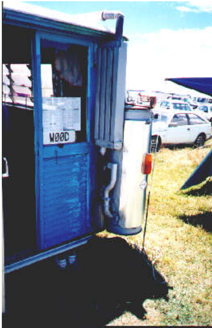
The gasified small bus with personalised number plate "Wood"
