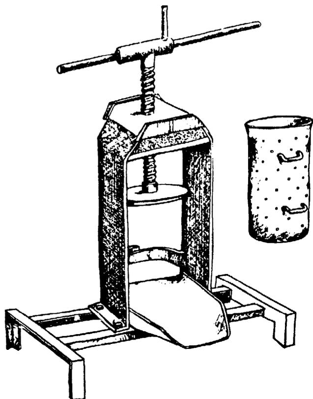
A hand-operated screw press is provided with 2 cages each of 17 litres capacity so that one can be refilled while the other is being pressed. Each reheated batch is divided into 3 pressing batches and each is then pressed for 10 minutes. The oil recovery by pressing is 90%.
