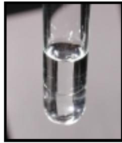
5{ ntaining blood (in .5 ml acetonitrile) are extracted for juvenile hormone (JH) by adding 1 ml hexane and 0.5 ml 0.9% NaCl solution. JH ends up mostly (about 98%) in the top hexane phase because JH is more fat soluable (less polar).
