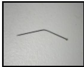
At least one insect pin, which is bent so that it is easier to orient to the bee body axis.
