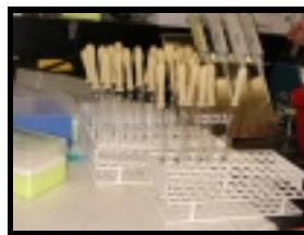
Each sample would have its own pasteur pipette (with a bulb) to avoid cross contamination.
