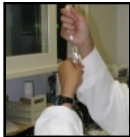
The hexane phase is easily removed by using a pipet.
