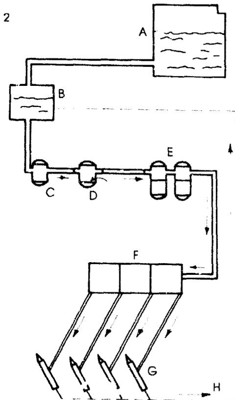
Fuel as received from the supplier is usually stored in a bulk tank, which should be situated outside the engine room. The main storage tank is normally made of steel and it is essential to make sure the steel is *not* galvanised internally, because all fuels are to a certain extent acid. Acid dissolves zinc plating, producing a gas that is highly explosive. It also leaves a sludge deposit in the bottom of the tank that could enter the fuel system, causing much damage.
