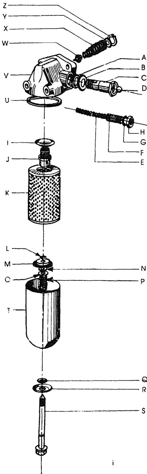
A typical oil filter assembly is shown in Fig. 1, in which the parts are:
