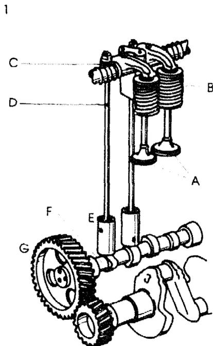
As you know, an engine must take in fuel/air and exhaust burned gases. Intake and exhaust must occur at precise intervals. Valves as shown in Fig. 1-A are used to do this job. The whole valve operating system is called the *valve train*:
