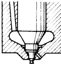
One way of improving this situation is to force the compression stroke air through a small orifice into a separate cell or combustion space, improving the swirling motion of the air.
