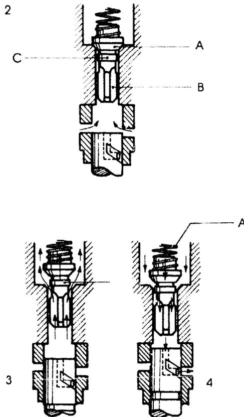
This pressure reduction is achieved by the construction of the mitre-faced delivery valve, see Fig. 2-A, fitted at the top of the pump body and by the flutes 2-B at the lower end of the valve. Just below the valve face there is a small plunger 2-C which has a very accurate fit in the bore of the valve guide. While the pump is actually delivering fuel to the cylinder, this plunger is raised clear of the valve body and fuel flows round it into the delivery pipeline, see Fig. 3.
