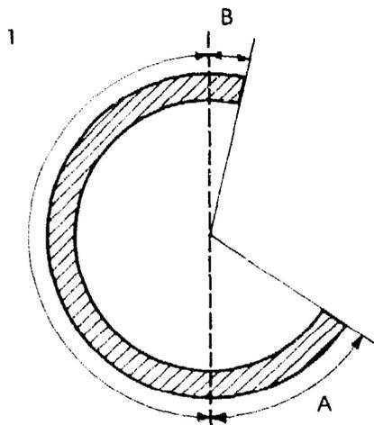
Figure 1 shows the diagram with degrees for the exhaust valve timing, where  $1-A = 65^\circ$  and  $1-B = 20^\circ$ . The exhaust valve opens at  $65^\circ$  before BDC (BBDC). The exhaust valve closes at  $20^\circ$  after TDC (ATDC).
