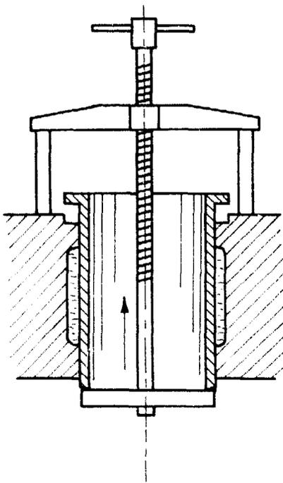
A cylinder is removed with a cylinder puller as shown in Fig. 1. After removing the cylinder the rubber or copper seals can be taken off. Then clean the counter-bores on top of the cylinder block and remove the scale from the water jackets with a wire brush. Also clean the lower sealing surface in the cylinder block where the rubber or copper seals are positioned.
