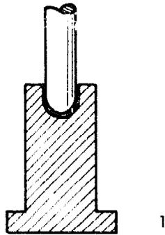
The movement of the cam is transferred by the tappet first, see Fig. 1. When the tappet is raised by the cam, some pressure is applied to one side of it, see Fig. 2. To enable the lifter to take this side pressure it is designed with a rather large diameter, see Figs. 1 and 2.
