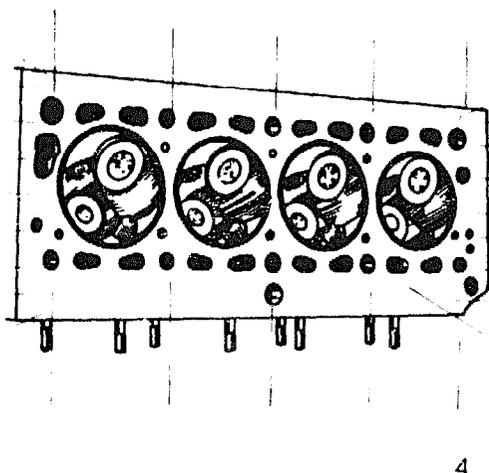
The cylinder head is fitted at the top end of the cylinder block and secured with studs or bolts passing through the head to the cylinder block. Most cylinder heads are cast from an alloy of iron and copper or aluminium. The intake and exhaust passages are cast or bored into the cylinder head as shown in Fig. 1:
