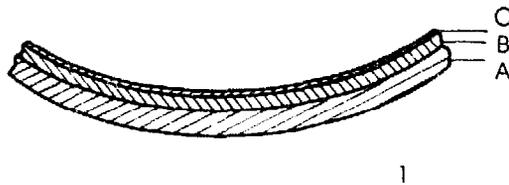
In general a bearing (see Fig. 1) has a body made of steel 1-A with some linings of different material 1-B and 1-C. The bearing material depends on the expected stresses.
