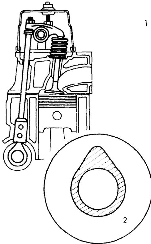
The camshaft is fitted into the engine block on the lefthand side, above the crankshaft, see Fig. 1. In small and medium sized engines it is generally made of a one-piece casting or forging and is supported by three bearings. Most camshafts are made of low-carbon alloy steel. The cam and journal surfaces are carburized before grinding them to their final shape.
