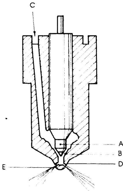
The multiple hole type nozzle in Fig. 2 uses a tapered valve 2-A which seats in a single orifice 2-B in the valve body. When fuel is pressed through the fuel inlet 2-C, it pushes the valve upwards and allows fuel to pass towards the spray tip 2-D and be sprayed through the nozzle holes 2-E.
