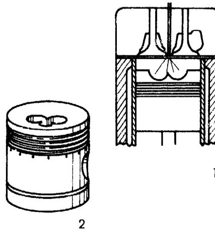
A turbulence chamber in the cylinder head is shown in Fig. 3. As you see, the fuel is injected into a small chamber in the cylinder head and shaped in such a way that it produces a highly turbulent condition.
