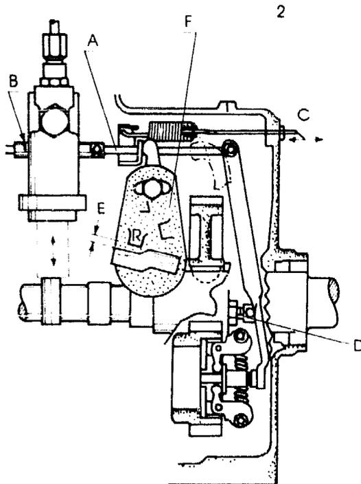
Adjust the governor lever fulcrum 2-D so that, when the calibration mark 2-B is against the outside of the fuel pump, the distance between the inside of the governor sleeve and the outside of the governor weight carrier complies with the manufacturer's technical data.
