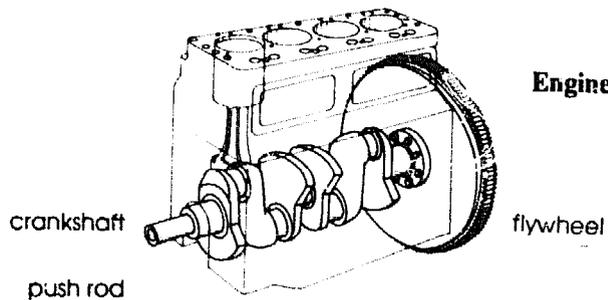
**Engine block: flywheel and crankshaft**
