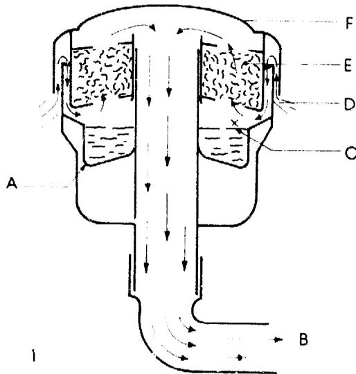
Figure 1 shows a cross-section of a light duty oil bath air cleaner. It consists of:
