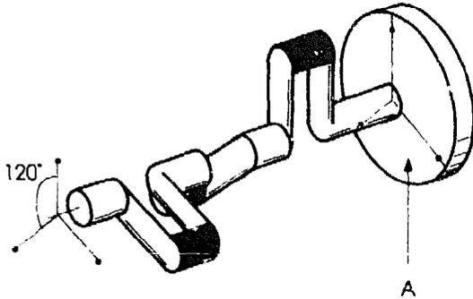
The power strokes thus follow each other more closely, resulting in a fairly continuous delivery of power to the crankshaft. For example, in a typical four-stroke cycle engine with three cylinders, the cranks are set 120° apart on the crankshaft, see Fig. 1.
