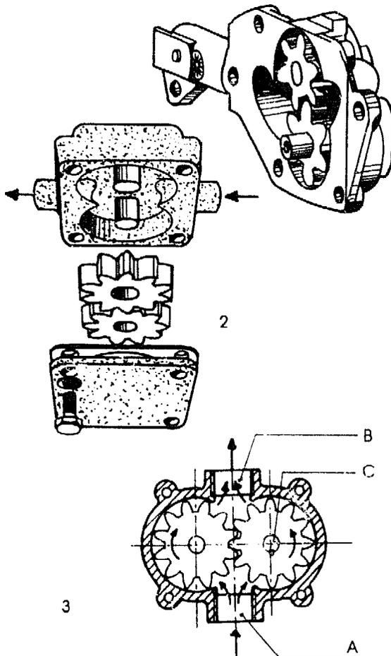
Gear pumps as shown in Figs. 1 and 2 are commonly used in diesel engines. They are either attached to the engine block as in the case of the pump in Fig. 1, or they are closed with a cover as shown in Fig. 2.
