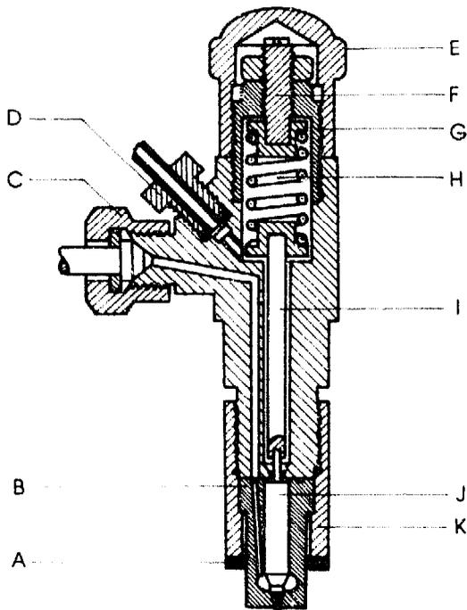
Injectors spray the fuel into the swirl chamber the moment the air in the swirl chamber has been compressed. Injectors consist of two principal parts:
