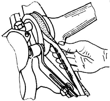
The demands made on the V-belt in connection with cooling the engine make it necessary to check the V-belt at regular intervals for signs of wear. The V-belt must be replaced if fibres along the sides become loose, see Fig. 1.
