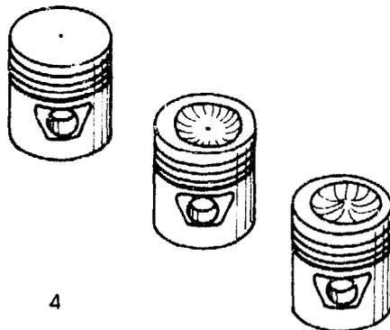
The piston is basically a plunger which moves up and down inside the cylinder. It seals off the crank case from the combustion chamber. Its main functions are:
