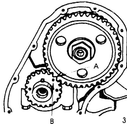
In some cases the two marks must match each other exactly, see Fig. 3. In other cases the punch dot on one of the teeth must match the other punch dot between the gearwheel teeth of the other wheel, see Fig. 4.
