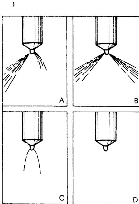
The primary function of a fuel injector nozzle is to atomize the liquid fuel so that it can be burned rapidly and efficiently in the cylinder of a diesel engine.
