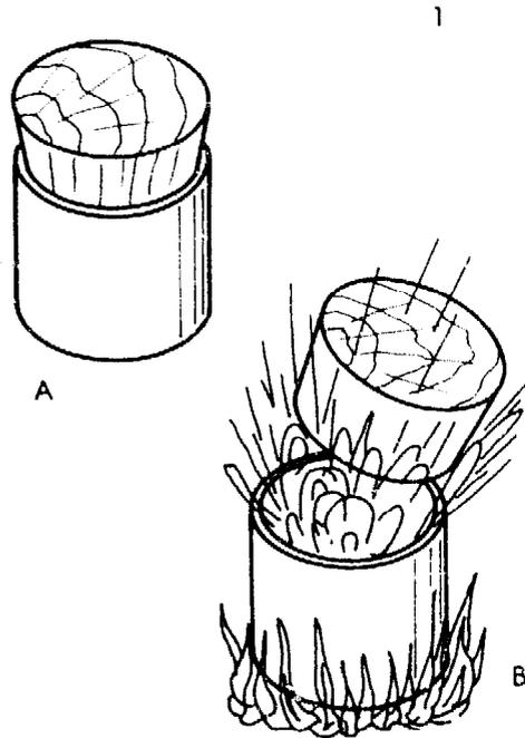
An internal combustion engine is an engine which burns fuel *internally*. This engine is basically a container, see Fig. 1, into which *fuel* and *air* can be fed and made to burn. Figure 1-A shows just such a container, closed with a stopper, in which there is a mixture of *fuel* and *air*. The mixture of fuel and air is highly flammable. If by any means the mixture is ignited, the container explodes, throwing the stopper out of the container with force, as shown in Fig. 1-B.
