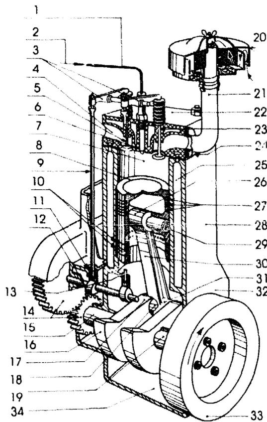
Figure 1 shows a section of a one-cylinder water cooled diesel engine. From the previous page you have learned the most important external parts. Now you have to learn the most important internal parts of the diesel engine.
