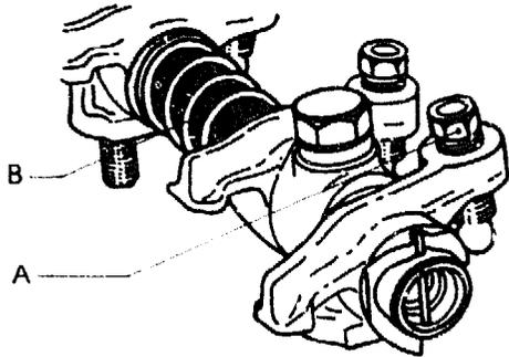
The rocker arm transmits the camshaft motion to the valves. The rocker arms shown in Fig. 1 are mounted on a hollow shaft 1-B which is secured with brackets and bolted to the cylinder head. Lubricating oil is pumped through the hollow shaft to lubricate all rocker arms. Springs are positioned between the rocker arms to keep them in place. A valve adjusting screw is shown at 1-A.
