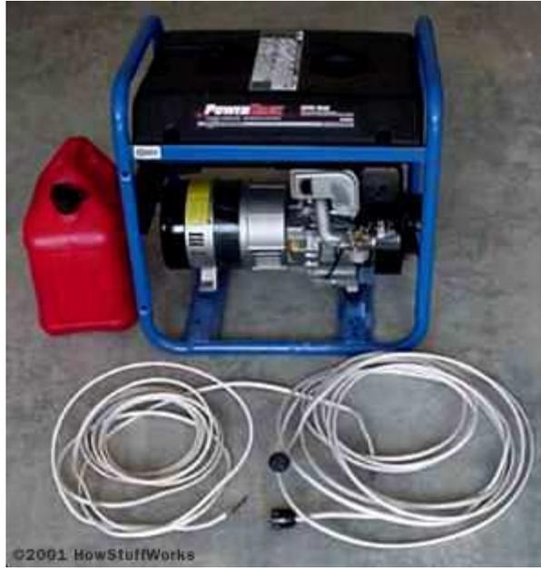
**A 5,000-watt gasoline-powered generator**
