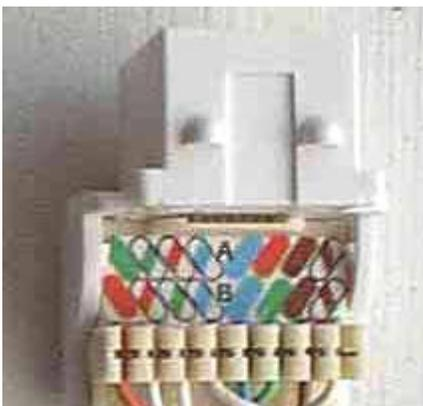
Jacks usually have punchdowns on the back or can be terminated without punchdowns using special manufacturer's tools or even a cover for the connector. Again, you **MUST** keep the twists as close to the receptacle as possible to minimize crosstalk.
