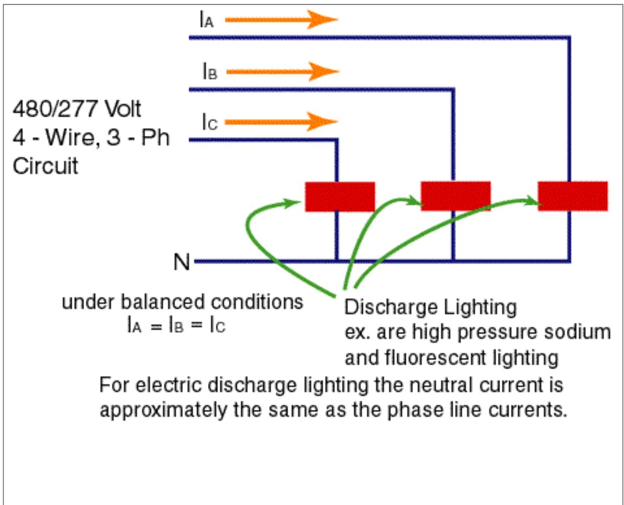
20. In the diagram below if  $I_a$ ,  $I_b$ , and  $I_c$  are equal to 50 amperes the current in the neutral is approximately \_\_\_\_\_ amperes.
