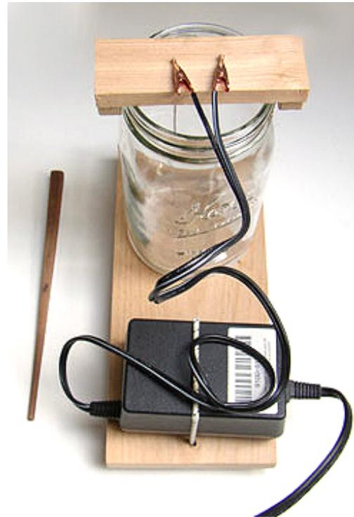
12. Plug in the AC adapter to wall outlet. You are ready to begin making colloidal silver solution.
