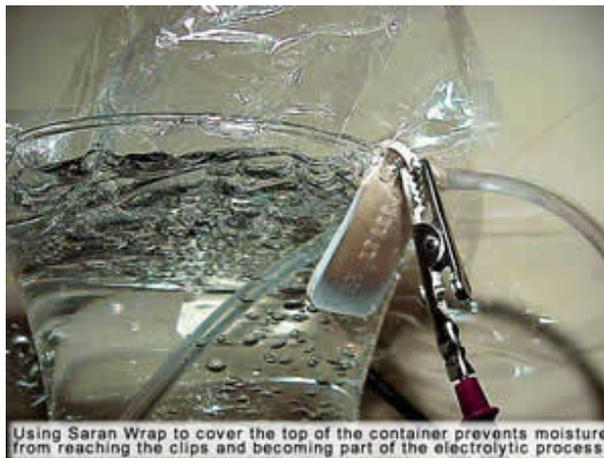
Using Saran Wrap to cover the top of the container prevents moisture from reaching the clips and becoming part of the electrolytic process
