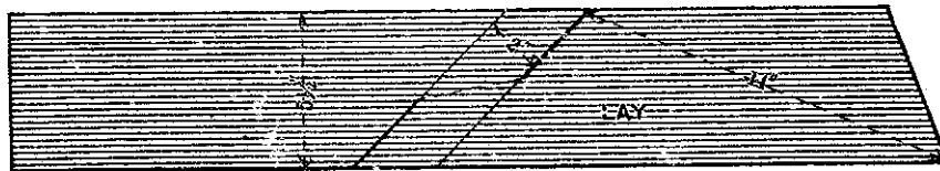
Making a Plow Lay. Fig. 318—Showing how to Mark the Steel.
