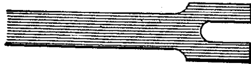
Fig. 62—Handle of Wrench Drawn Out.
