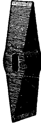
Fig. 1—Hatchet for Opening Bundle Iron. Made of 1\frac{5}{8} square Steel.
