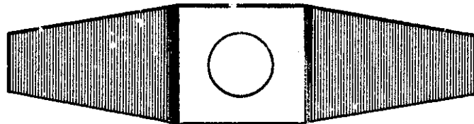
Fig. 284—Showing how the Ends are Drawn.
