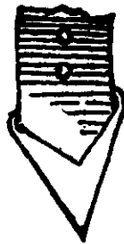
Fig. 389—The Point Adjusted Ready for Welding.
