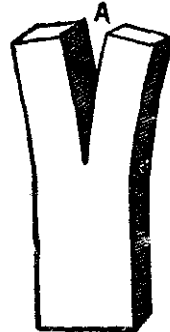
Making a Step-Leg. Fig. 186—Showing how the Iron is Split.
