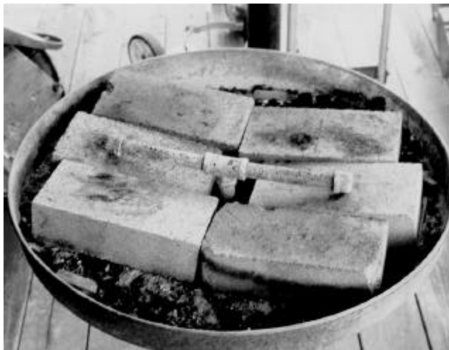
Placement of the bottom bricks and tuyere
