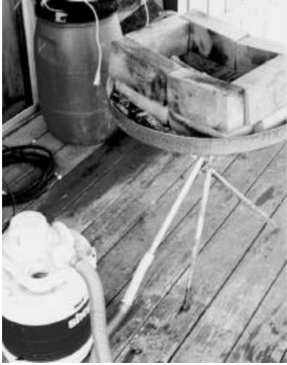
Assembled forge with shop-vac
