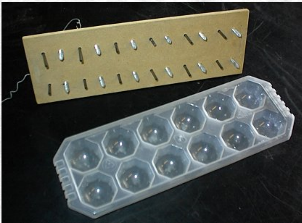
Figure 2. The multiple pairs of electrodes are shown attached to the wooden support. This is the 'high' voltage, 'low' current version. The ice cube trays hold the electrolyte for each cell. The cells are wired up above the board.
