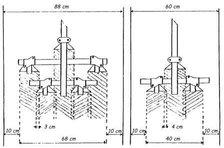
Figure 46: Arrangement for five times (left) and three times (right) to work with a single pass in row widths of 90 and 60 cm respectively.
