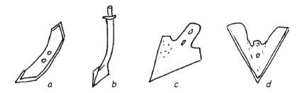
Figure 36: Several examples of a scarifier tine: (a) The reversible point for scarifying harder soils. (b) The rigid point. (c) The duckfoot point for scarifying lighter soils and general weeding operations. (d) The sweep used for weeding.
