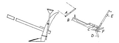
Figure 43: Simple hand-metered tube seeders. "Nan" single-row seeder used in India (left) and a simple seeder-weeder developed in Sudan (right).
