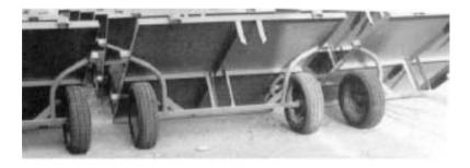
Figure 28: Two-wheel carts using roller bearings and factory-reject car tires. Designed for a team of oxen, but a smaller size is used with donkeys in Togo.
