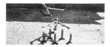
Figure 37: The Houe Manga in this illustration has the four lefthand tines correctly alligned. The right-hand tine, however, needs adjusting.
