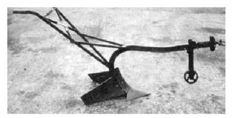
Figure 42: The Agrimal ridging plough weighs 44 kg; the wings are adjustable.
