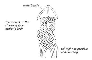
Figure 19: Harness made out of braided goatskin. Any number of leather strips can be used but even numbers are easier.
