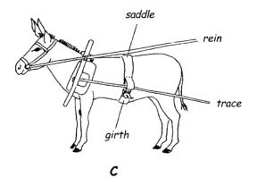
Figure 21: Three-pad collar harness with saddle and girth.
