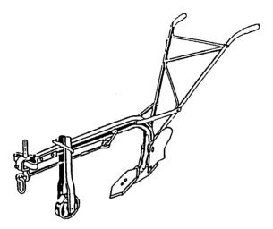
Figure 38: Magoye ripper attachment on plough beam.
