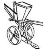
Figure 44: Ripperplanter attachment to the common plough.
