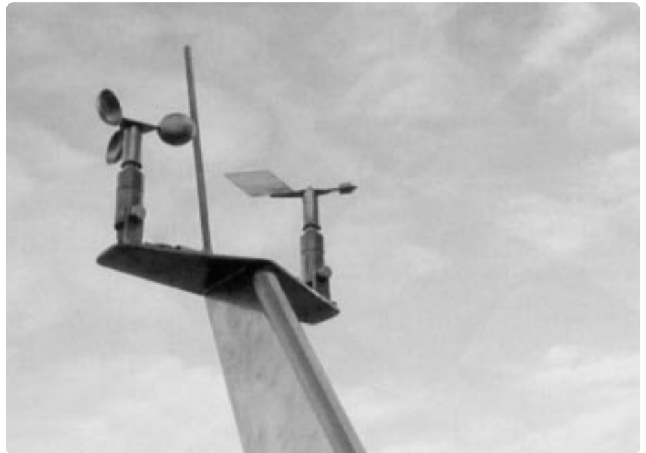
Cup anemometer for wind speed indication (left) • Lightning conductor (middle) • Wind direction indicator (right)
