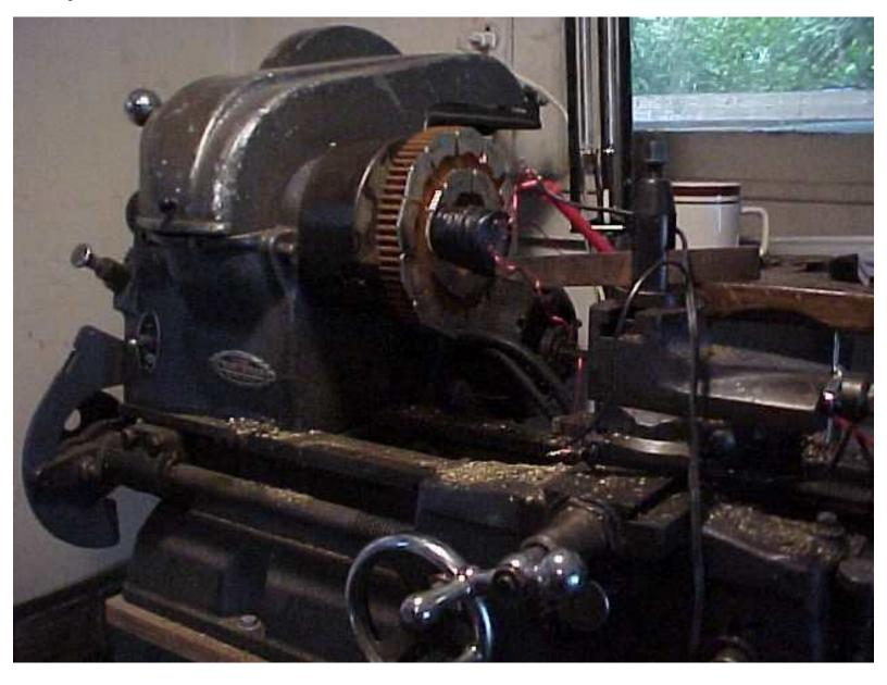
Next step was to turn it on, and test the different taps on the coil, at 3 different speeds. I used a 12 Volt, 5 watt light bulb as a load, and tested the voltage of each tap on the coil, at each speed, with, and without the load. The tests were done at 200, 400, and 600 RPM.
