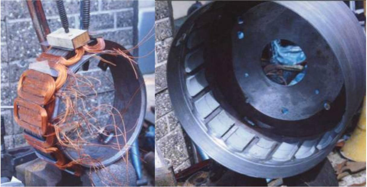
The 20 magnets used are also neodymium ones, with a rather unsuitable curve on them, but they are nicely fitted to the rotor by painstaking machining.
