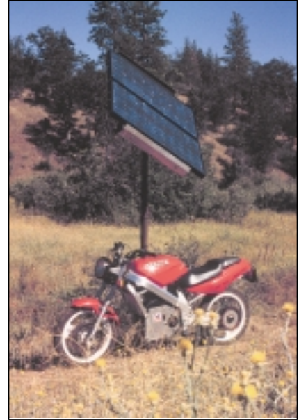
Solar panels recharge an electric motorcycle miles from grid power.
