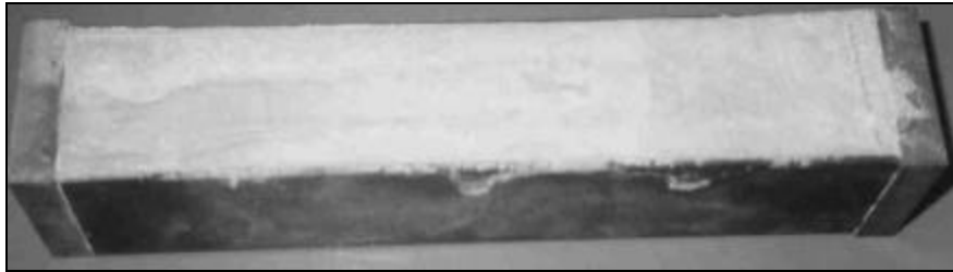
Figure 5.15 Micro crack development in restrained sample
