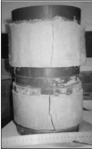
Fig 5.25(a) Polypropylene fibre reinforced
