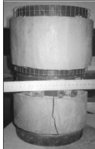
Fig 5.25(c) Square mesh reinforced
