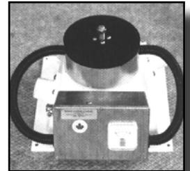
ES&D hydroelectric battery chargers use a cast bronze turgo runner to drive a long-life, brushless permanent magnet alternator. A simple change of wiring in the junction box allows this turbine to charge 12, 24, or 48-volt battery systems. These turbines come with cut-to-size nozzles that can be user-set for up to 1", allowing a very large flow in low head situations. They can operate on heads as low as five feet with a flow of 40 GPM.
