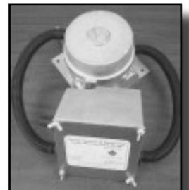
This new tiny turbine, a miniature version of the Stream Engine above, is ideal for sites with good head, but with very little flow. Two models are available; one for 12 to 48 volt charging and one for high voltage transmission. At 3 GPM and 100 feet of head, the Waterbaby will charge at 25 watts.
