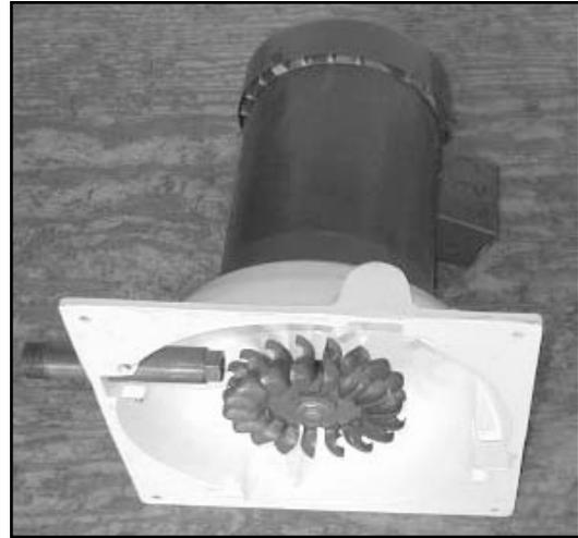
HI-Power Hydroelectric generators are ideal for sites where water is far from power needs (up to 10,000 feet), or when greater power is required. High transmission voltage can be sent over a mile before being 'stepped down' to battery voltage. It comes complete with step down transformer, rectifier, fuses and amp meter. Use a diversion type regulator with these units.
