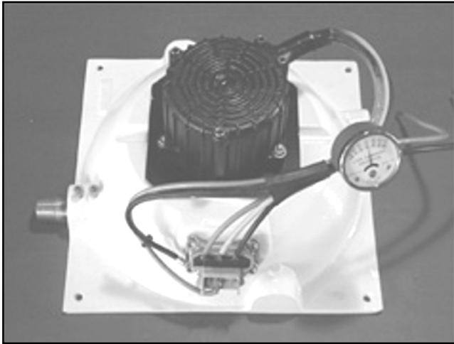
Hi Power is now offering a low voltage brushless PM generator. This user-friendly unit requires no adjustments and is more efficient than car alternator types over a wider range of head and flow.
