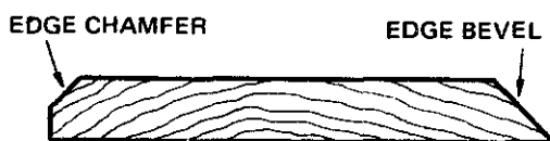
Fig. 8-38 Comparing a chamfer to a bevel.
