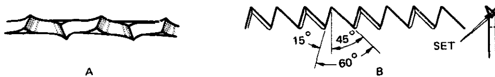
Fig. 7-25 How teeth should appear when completed.
