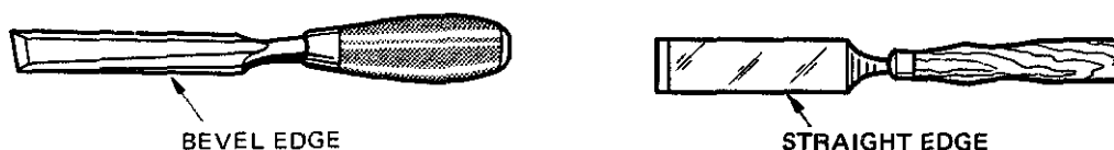
Fig. 9-10 Wood chisel blade shapes.
