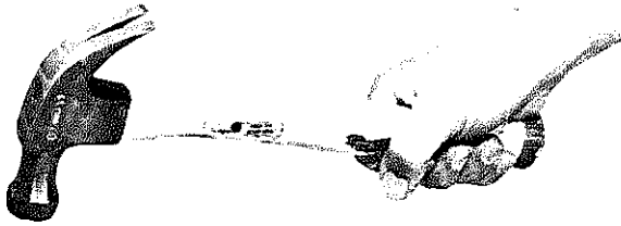
Fig. 11-24 Correct method of holding a hammer.
